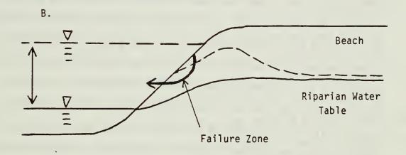
Figure 1: Concept of beach erosion. A. Tractive force erosion;
