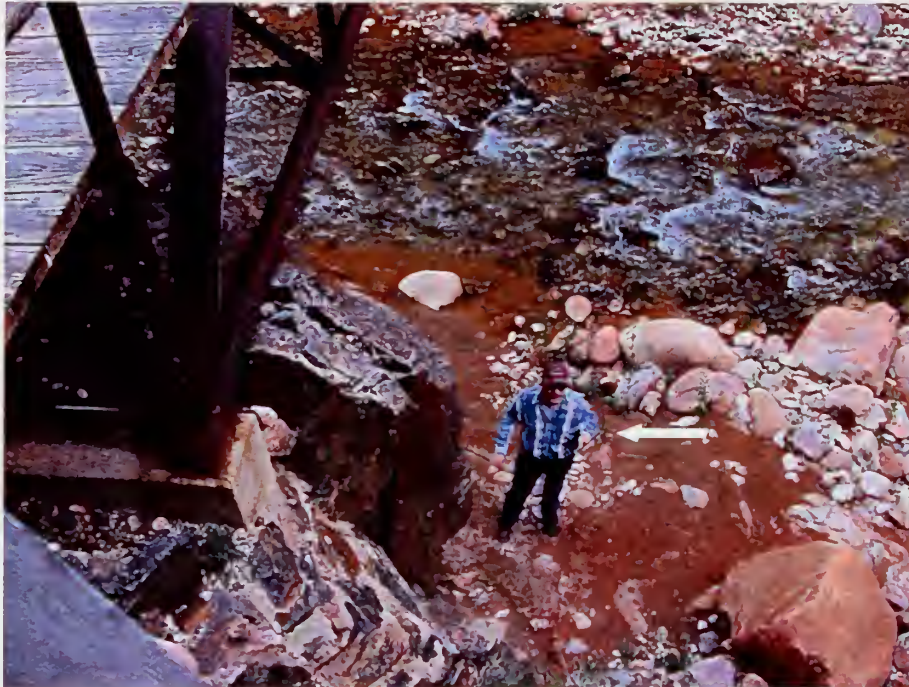
Figure 3. Anode 7 at pipeline stationing 242+30. Anode cable has been severed (arrow) and appeared to have been severed for some time. It is speculated that the anode cable was severed by the buildup of debris on the cables during flash flooding.
