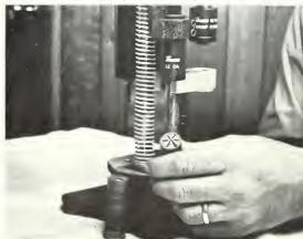
Slide the shell from the crimp starter position to the final post. Press the lever down, and Presto! A perfect crimp and a fine load, tailored especially for the kind of shooting you want to do.
