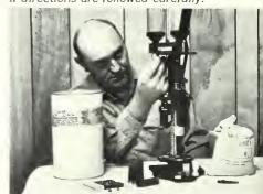
The bushings are put into place in the charge bar of the reloading press. Make sure the shot bushing is under the shot holding tube, and the powder bushing is in its proper place under the powder reservoir. Reversing these two would be dangerous.
