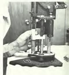
The third station performs several functions. First, depress the lever to insert the loading tube into the hull. Slide the charge bar to drop the powder charge. Bring the lever up, insert the wad column, and press firmly to get the proper pressure on the wad (refer to reloading manual for correct pressure.)
