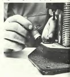
The new primer is placed into the seating die on the second station, the hull is placed on top of the primer, then pressed onto it to seat the new cap into the pocket.
