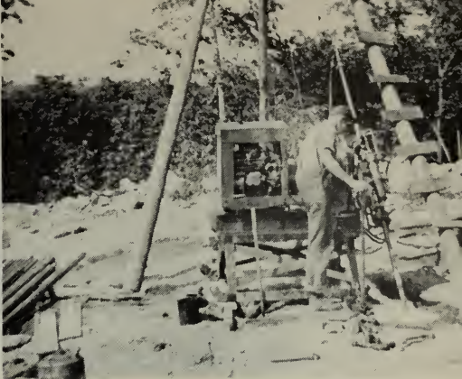
Detailed exploration by diamond core drilling is uncovering large reserves of pyrophyllite and other refractory minerals.
