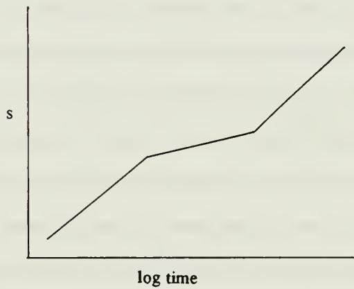
Figure 49. Configuration of aquifer test plots with varying transmissivity and storage values.
