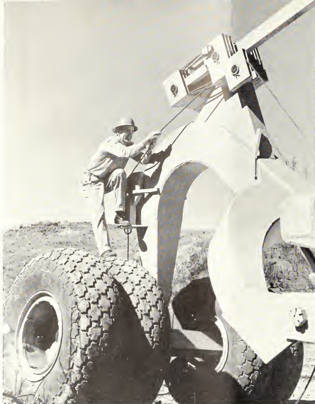
Workman strings cable through operating mechanism of 28-cubic-yard scraper used in excavation
