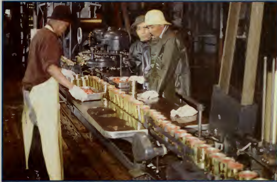
"Canned fish weighted and patched before lid and salt added," courtesy of Dorothy Fribrock, private collection.
