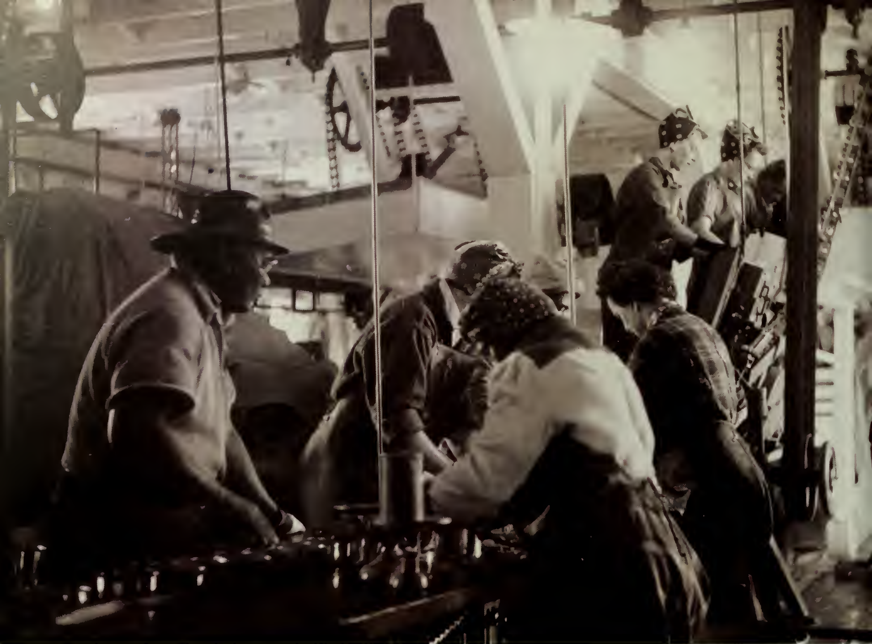
"In the foreground is the 'patch table' where small pieces of salmon are inserted in cans imperfectly filled by machinery," The Alaska Sportsman, August 1953.
