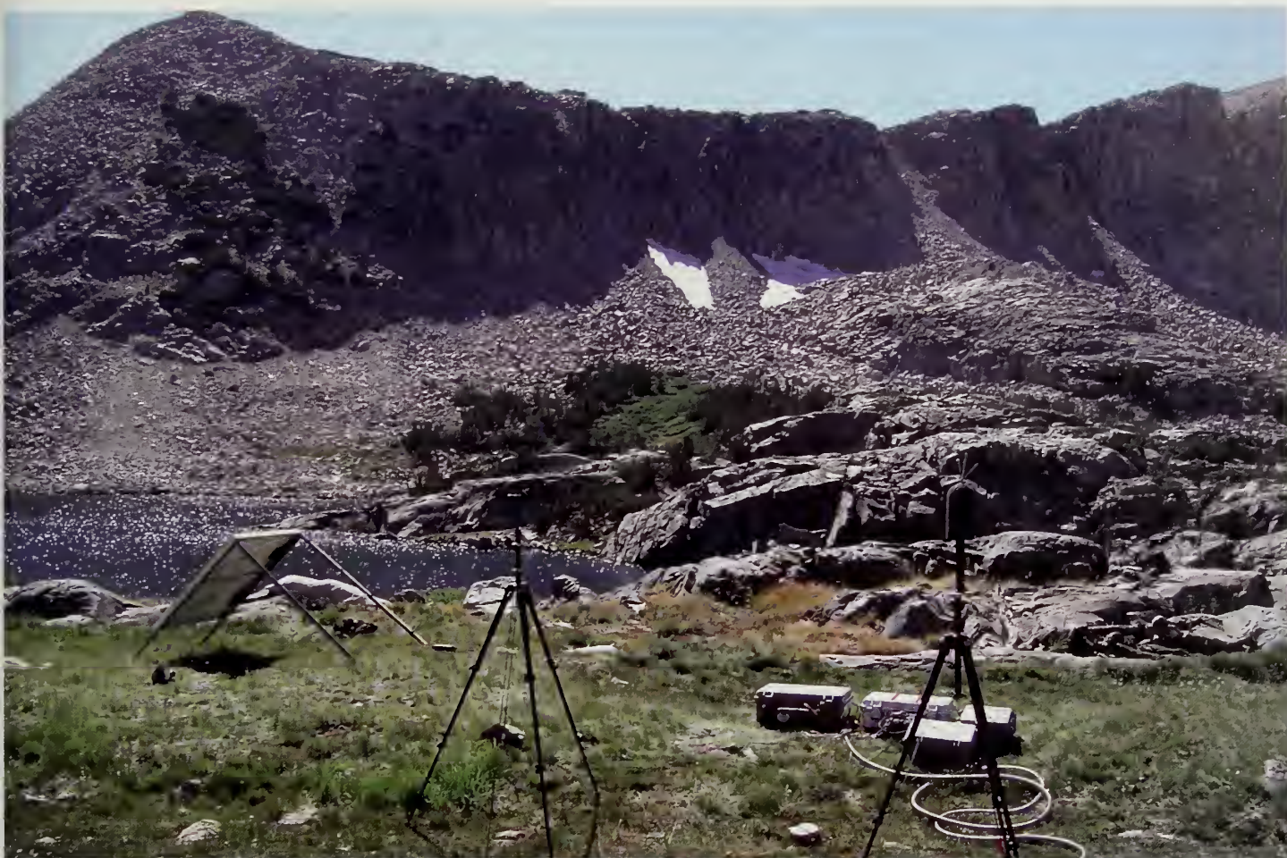
Automated acoustic monitoring system at a high-country site at Yosemite National Park.
