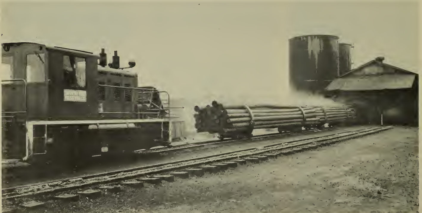
MORE POLES FOR SOUTH'S EXPANSION —A charge of freshly-creosoted Southern Pine poles leaves the treating
