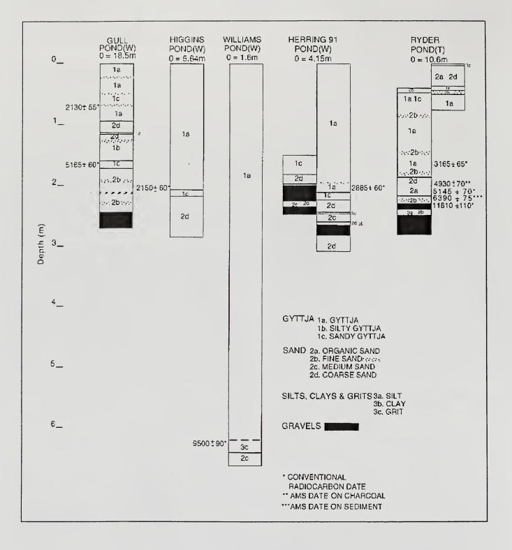
Figure 2-2. Sediment stratigraphy, radiocarbon (yr B.P.) and 210Pb (A.D.) dates, for the pond sediment cores referred to in this chapter. Note depth scale change from meters to centimeters for Snow and Long ponds. Refer to legend (1a., 1b., etc.) for sediment type changes. W = Wellfleet, T = Truro.
