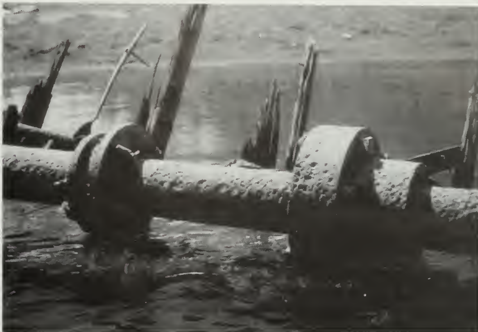
Figure 5.37. Top view of propeller shaft bearing. Scale = 1 foot. NPS photo by Brett Seymour.
