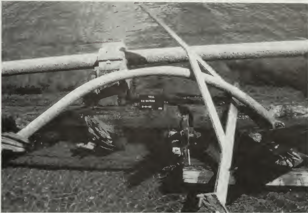
Figure 5.49. Davit (left) and support bracket (right) within E. C. Waters ' wreckage. NPS photo by Brett Seymour.
