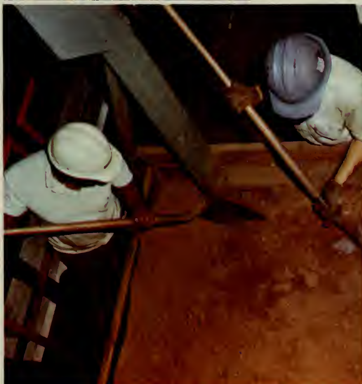
(Middle) Chemicals are used to make the valuable particles in the crushed ore clump together. Waste materials are removed by "desliming." (Left Bottom) Nonmagnetic taconite iron ore, being prepared for metallurgical experiments, was considered useless until the Department's Bureau of Mines developed a practical technique for converting it to high-grade iron ore concentrates. Billions of tons of taconite are found in Michigan and Minnesota. (Right Bottom) Waste minerals are removed in the froth overflowing the flotation cell, and the iron-rich concentrate is collected from below.
