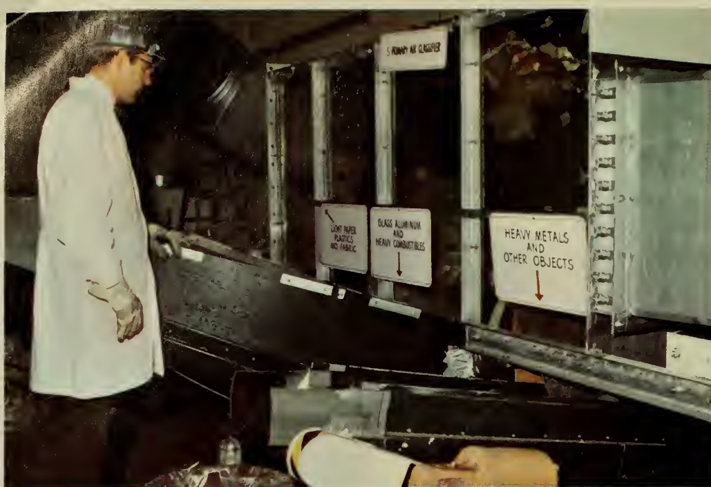
(Top) The experimental Bureau of Mines process for separating useful raw materials from unburned trash and garbage uses "air classification," which works on the ancient winnowing principle. (Middle) A special optical separation technique, used in the Bureau of Mines experimental trash recovery plant, separates crushed glass into clear and colored "fractions." (Bottom) The trommel, a standard item in many ore-processing and coal-sizing operations, is proving useful in trash recycling research. (Right) Relatively clean scrap paper in the bags is one product of the experimental recycling facility for "raw" urban refuse. A large-scale plant operating continuously could produce a steady stream of reclaimed paper in large enough volume for recycling by industry or use as clean fuel.
