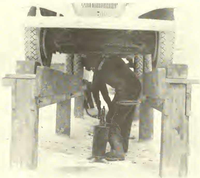
ELEVATED GREASE RACK USED BY C. C. C. INSTEAD OF DANGEROUS GAS-COLLECTING GREASE PITS
