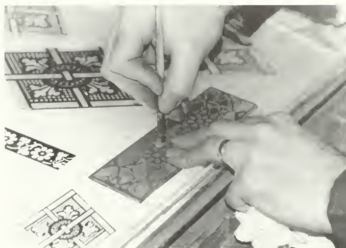
Figure 15. New stencils are used to produce matching replacement glass for repetitive stenciled patterns in a ca. 1870 window. Photo: Neal A. Vogel.
