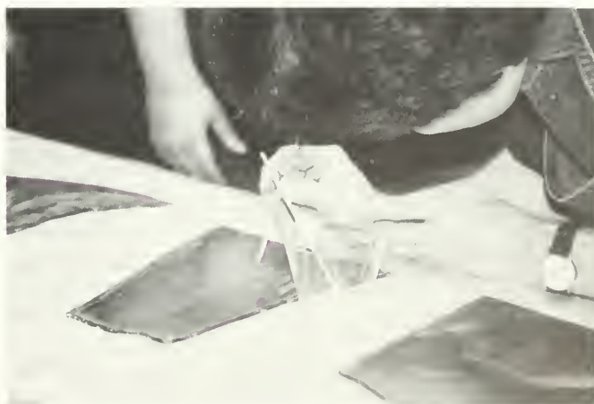
Figure 17. A valuable piece of flashed glass is carefully edge-glued with epoxy and a steady hand. Photo: Neal A. Vogel.
