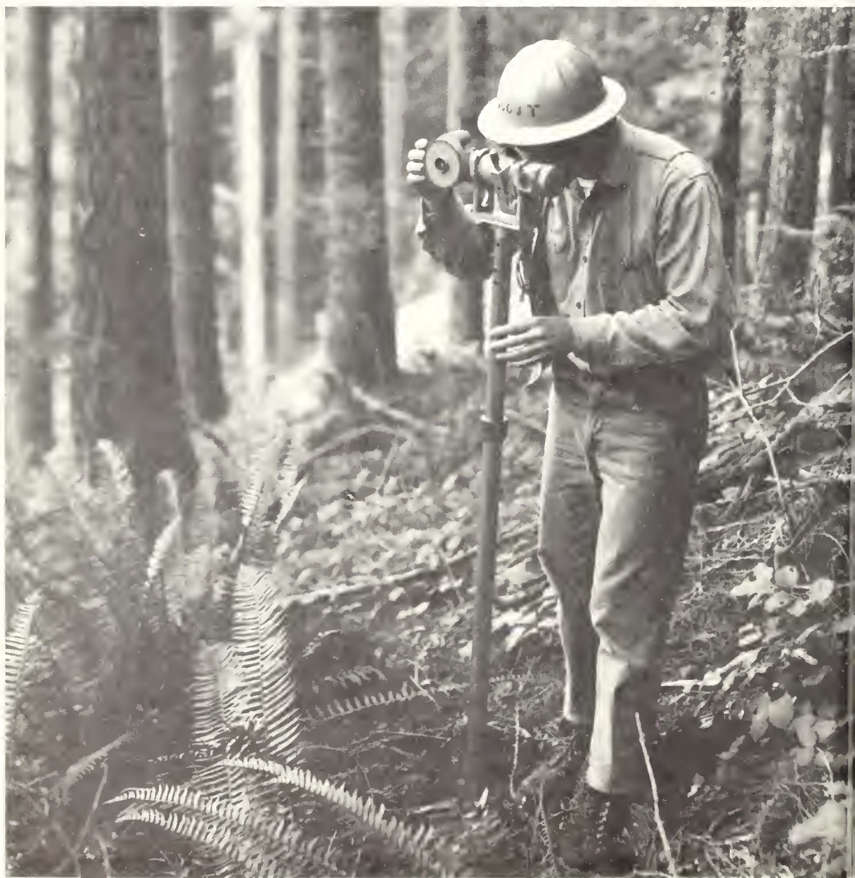
Figure 4.--Optical dendrometer used to measure upper-stem diameters and heights on standing trees.
