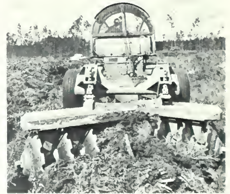
This bedding harrow is preparing cut-over and cleared woodland for planting of pine seedlings.
