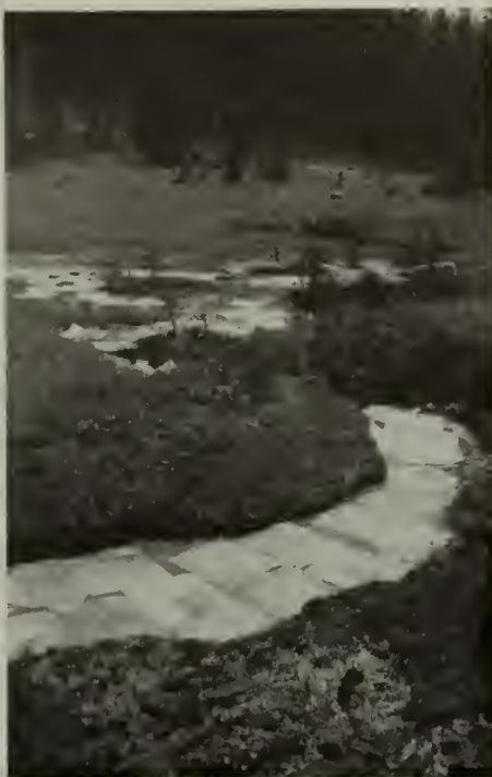
Doing their thing , these white "diapers" sop up spilled oil without absorbing water in Paradise Meadow.
