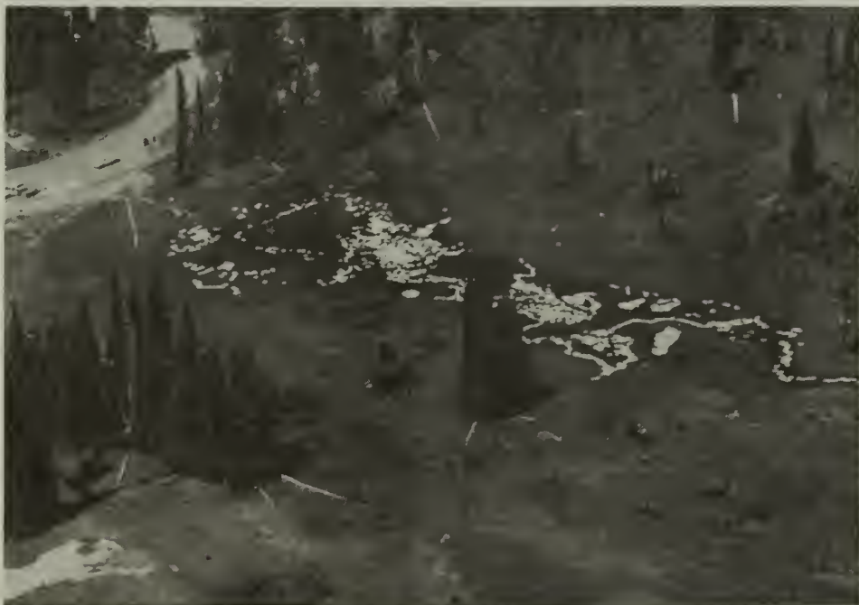
Aerial view of Paradise Meadow shows parking area at far left, oil draining in at top left-of-center, and oil draining out at right just below center (into Paradise River). The white patches are some of the several thousand absorbent pads used to soak up oil. Dark areas are dead or dying vegetation.
