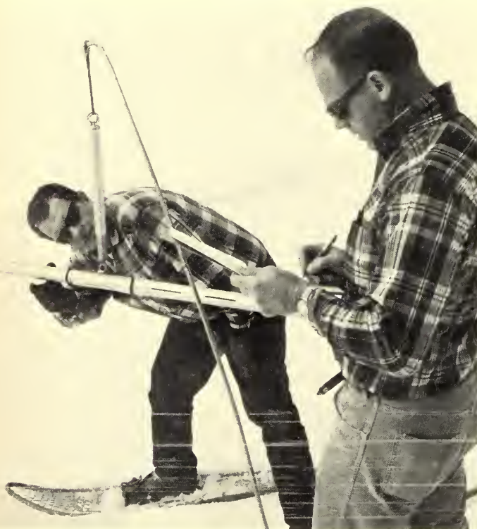
Salt River Project employees, Ken Vineyard, left, and John Wescott, check weight of snow in tube to determine the quantity of moisture in the snow—this helps the project predict potential runoff.
