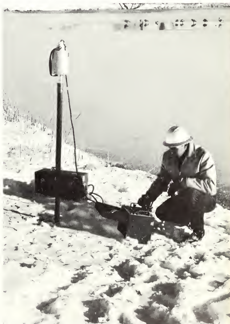
Looking much like a parking meter is the Bureau's much-used nuclear moisture probe. Resting atop the pipe is the heavy protective case made of lead. The supporting pipe is for lining test holes in the ground. B. A. Callow is a technician from a Reclamation unit at Denver, Colo., who is demonstrating the instrument, typically, near a body of water.
