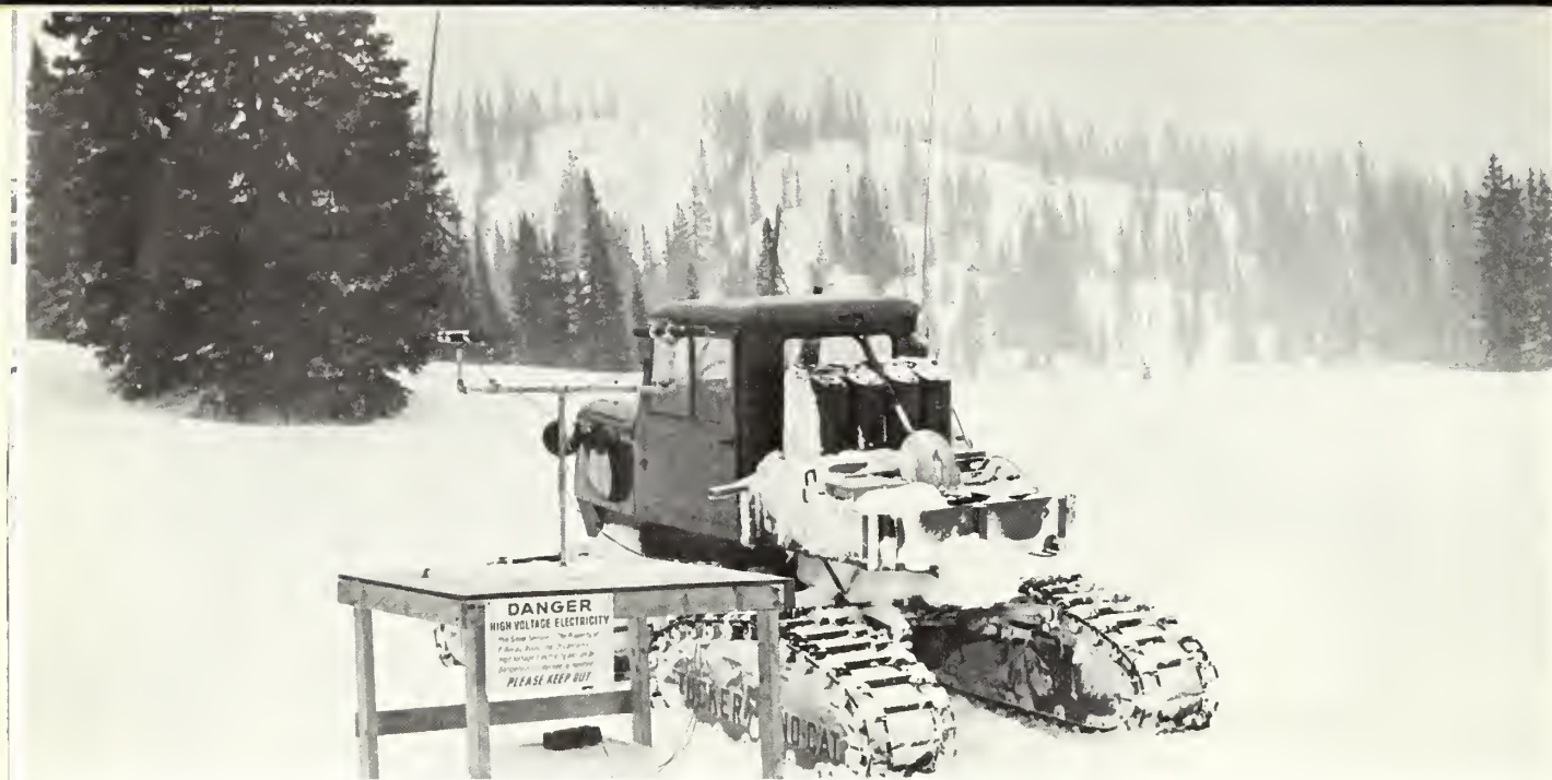
Specialists in atmospheric research cover difficult terrain by wide-track snow vehicles in order to check snow-rate measuring instruments (one in foreground) at isolated stations.
