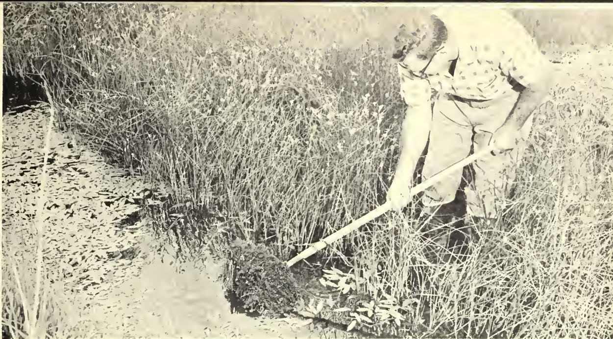
A plant specialist is shown examining a weed test in an experimental irrigation lateral at the Denver Federal Center.
