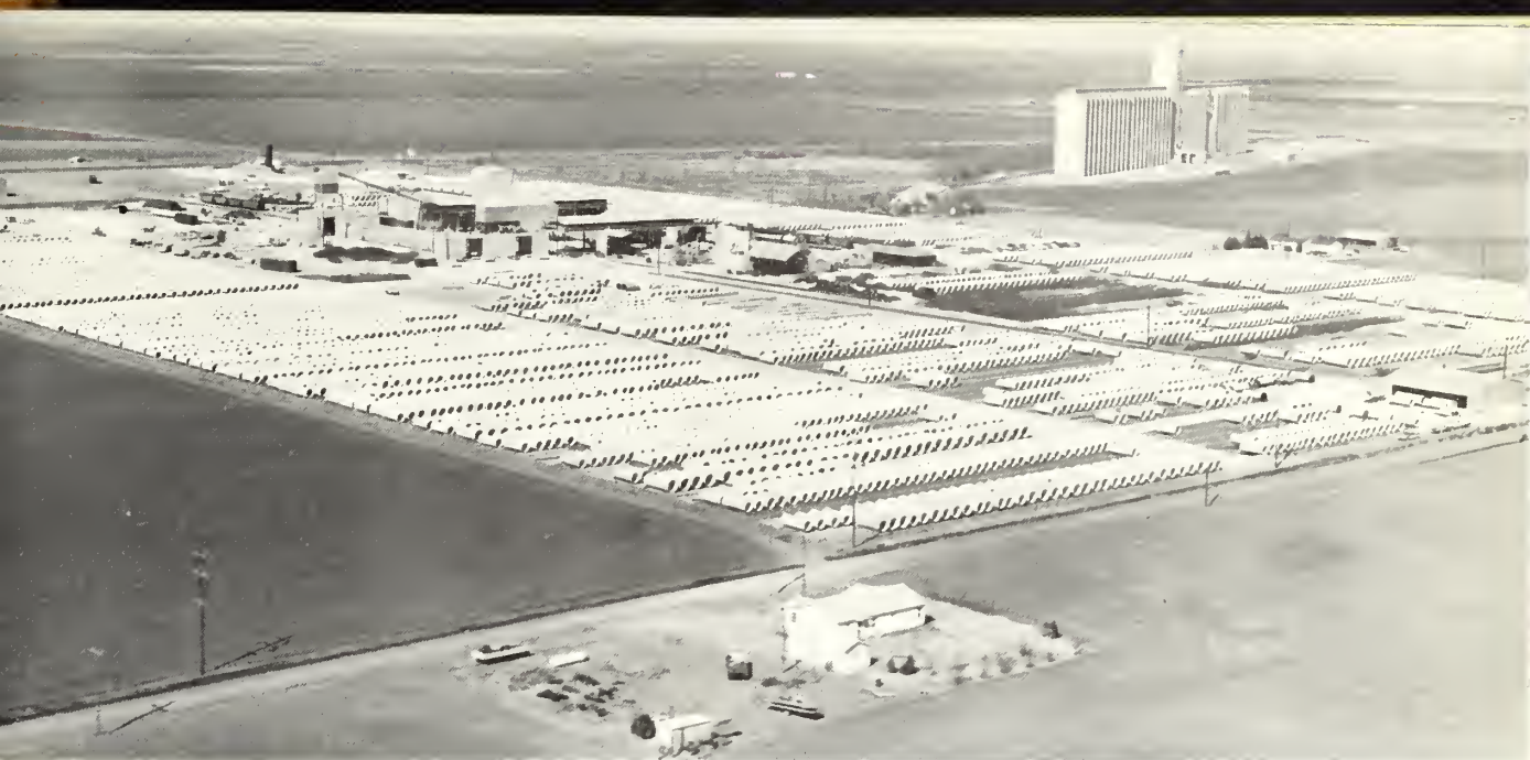
Row upon row of large concrete pipe at this manufacturing plant and storage yard of Cen-Vi-Ro of Texas, Inc., near Plainview, were stalled in the 322-mile aqueduct.
