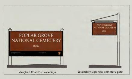
signs, the new signs should employ a contemporary, compatible design using a rectangular board, simple symmetrical layout, and an upper case font. Design the Vaughan Road entrance sign as the primary (larger) sign, and the one near the entrance gates as a secondary, more subtle sign in deference to gates (fig. 4.6). Remove the non-historic stone ring and planting bed around the Vaughan Road sign and maintain the foreground as lawn.
