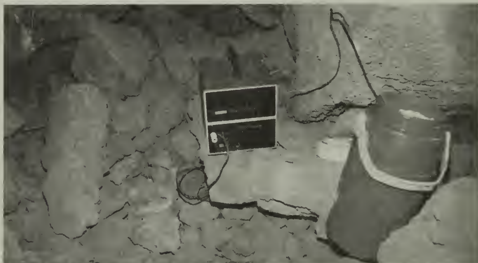
Temperature indicator shown here is reading a thermocouple imbedded in cave rock. The ice bucket is used to calibrate each thermocouple reading.
