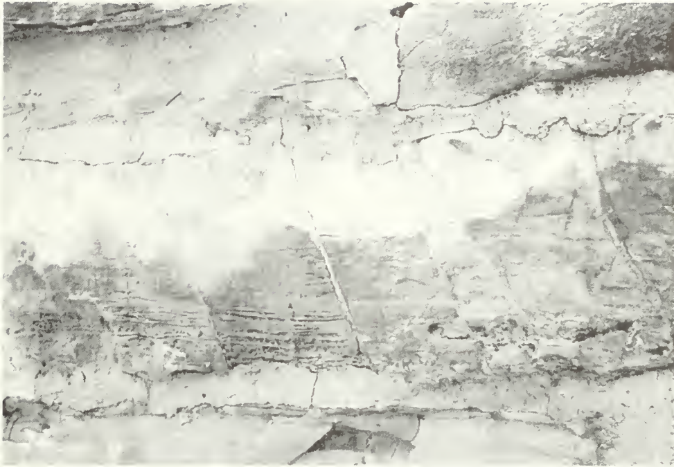
Figure 115: Red color of limestone caused by excessive heat.
