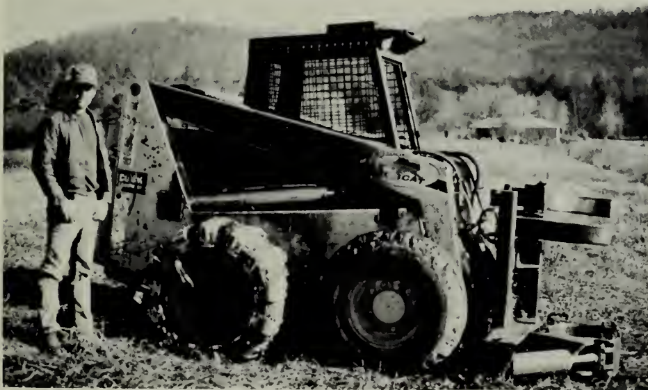
Figure 1.--Bobcat feller-buncher used on shear plots. Notice the tracked rear wheels which were thought to be very damaging to small stumps.
