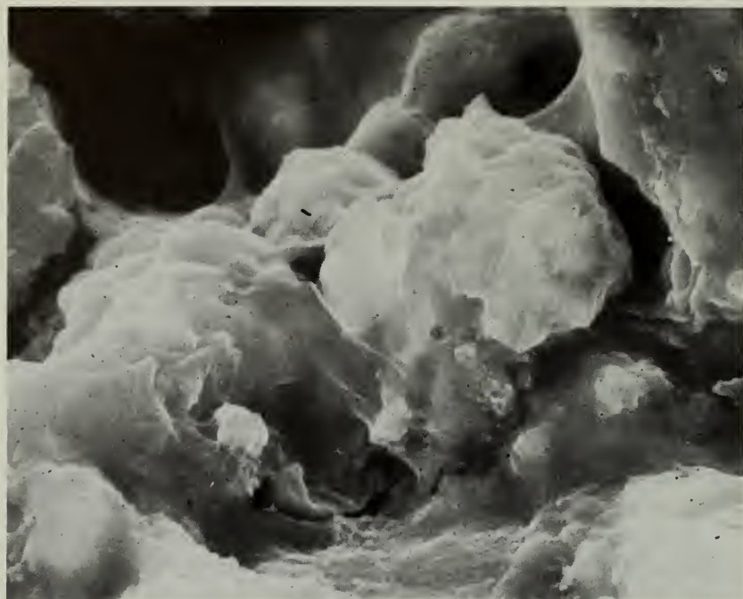
Fig. 3. Scanning electron microscope photos (SEM; \times 20,000 ). Amorphous \text{Fe(OH)}_3 is the only Fe mineral on the surface of alluvial fan.
