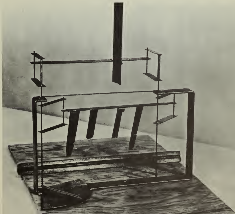
Reproduction of lift balance used in 1901 wind tunnel; model airfoil in testing position. The original balance is in the Franklin Institute.
