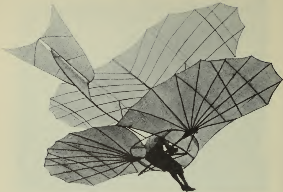
Lilienthal's two-surface glider of 1895 in which some of his highest and longest glides were made. This German engineer made hundreds of glides with various apparatuses employing birdlike wings.
