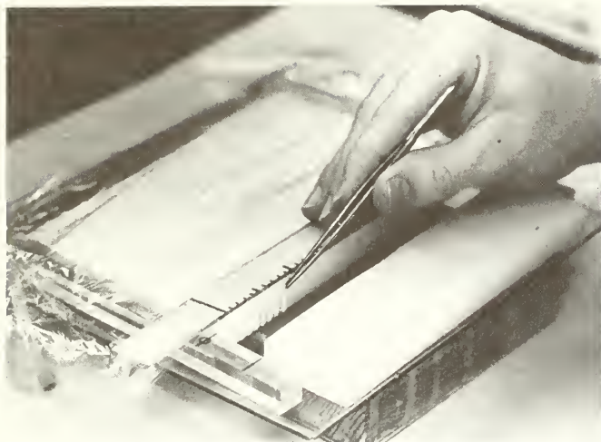
Figure 5 —Cut gel surface open at the origin. Wicks containing the absorbed liquid fraction of samples are placed on the vertical surface in order corresponding to their listing on the data sheet.
