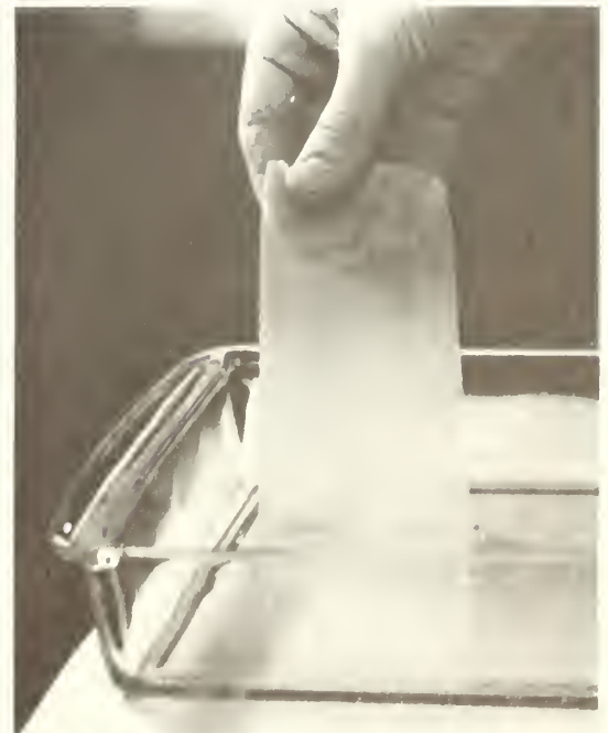
Figure 8 —Gel is prepared for slicing by using plastic spacers attached to the glass on either side of the gel slab with spring loaded clips. Above: taut monofilament nylon sewing thread cuts horizontal slices through the gel slab. Right: gel slice is placed in an appropriate stain solution.
