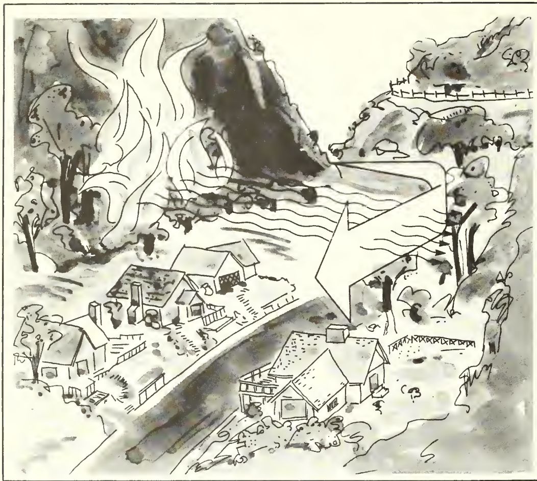
Figure 17 —Radiation transfers heat in all directions—even against a wind sweeping through a canyon. In the process, the hillside opposite a burning slope can be ignited.
