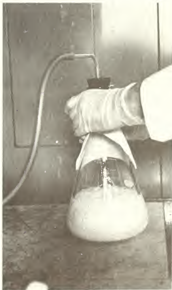
Figure 4 —Degassing hot starch using vacuum line attached to a cork in the top of the vacuum flask while blocking side port of the flask with a finger.
