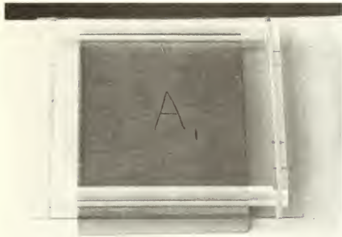
Figure 2 —Gel mold consisting of plastic bars secured with rubber bands to single strength window glass.
