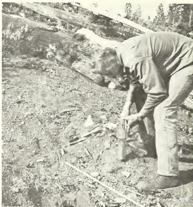
Figure 6—Movement of radio-tagged seeds is traced with a scintillator.
