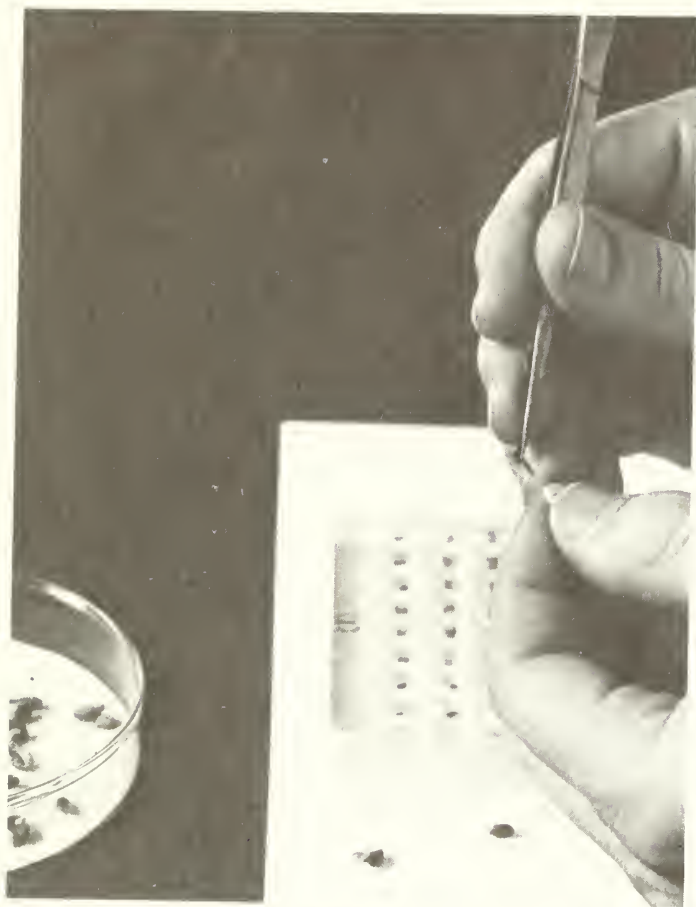
Figure 1 —Sample preparation materials. Left : germinated seed in the petri dish used for germination, and a dissected seed with gametophyte and embryo. Above : grinding block, 8.5×8.5×1.3 cm clear plastic with 0.7-cm holes (1/4 inch) drilled 1.0 cm deep (flat bottom holes were drilled with a bit squared off on a grinding wheel), placed on a frozen pad of Blue Ice for cooling (grinding block and pad were frozen together before samples were loaded into the holes). Below : data sheet with the identity of the samples coded to the numbered holes in the grinding blocks.
