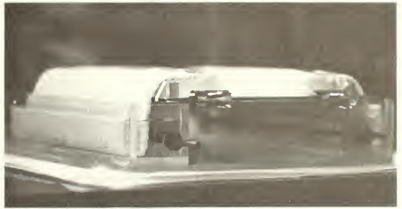
Figure 7 —Side and top views of an electrode tray with gel and wicks, sponges, and plastic wrap in place.
