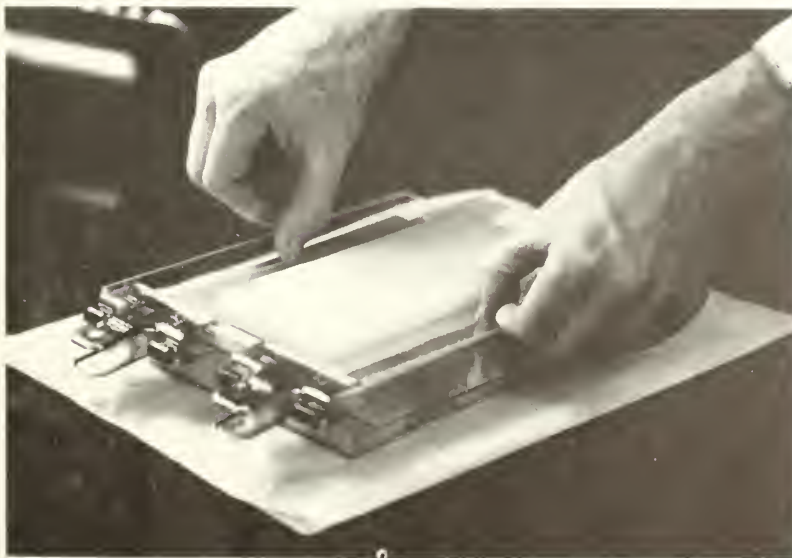
Figure 8 —Gel is prepared for slicing by using plastic spacers attached to the glass on either side of the gel slab with spring loaded clips. Above: taut monofilament nylon sewing thread cuts horizontal slices through the gel slab. Right: gel slice is placed in an appropriate stain solution.
