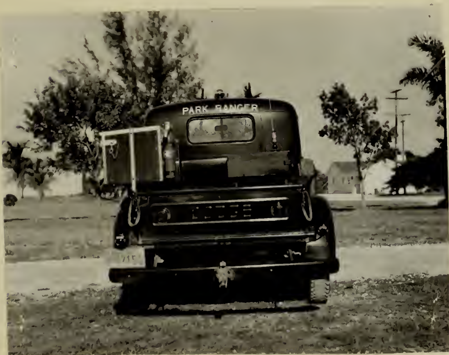
REAR VIEW Showing Location of Box, CO 2 Fire Extinguisher, Radio, Lights, Trailer Hitch, etc.
