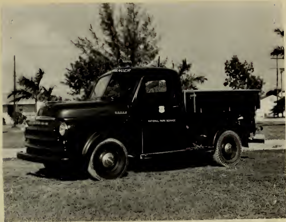
SIDE VIEW Showing Location of Box, Siren, Lights, etc.
