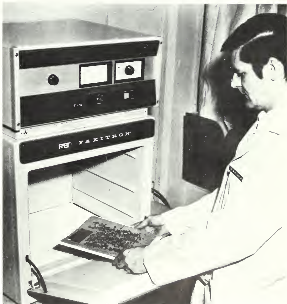
Dr. Earl W. Belcher, Jr., director, Eastern Tree Seed Laboratory, places tree seed in the x-ray unit. Through the x-ray he will be able to determine the amount of insect and mechanical damage and seed development. The x-ray does not affect germination.
