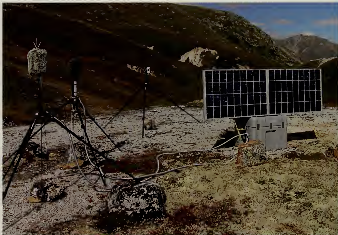
Sound monitoring station at Hidden River, on the South side of the Alaska Range in Denali National Park and Preserve. Improvements to recording equipment resulted in 60 percent less power consumption.
