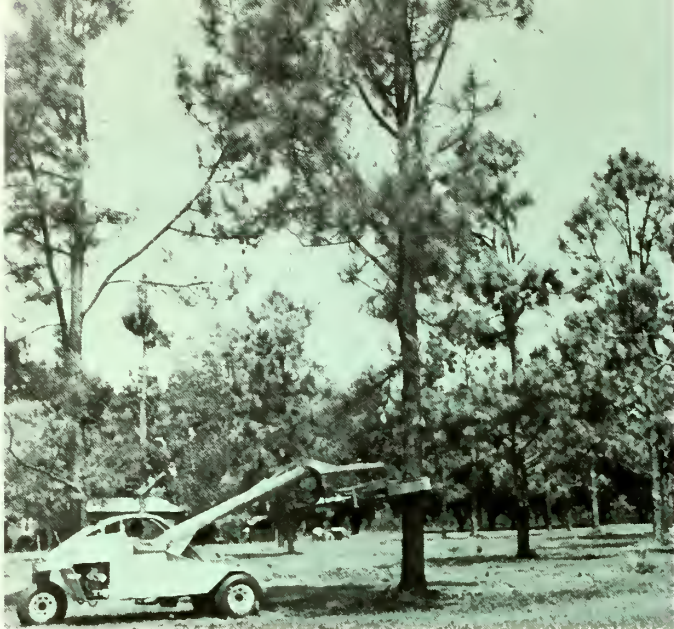
SHAKER LOOSENS PINE CONES
