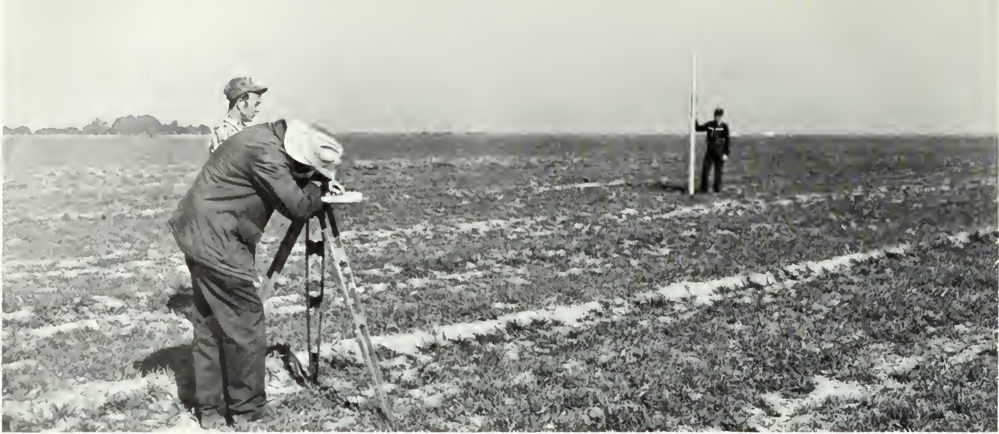
Jimmy O. Lowther of Hinesville, a civil engineer technician with the Soil Conservation Service, operates an alidade on a plane table to plot a contour map of the Commission's new
