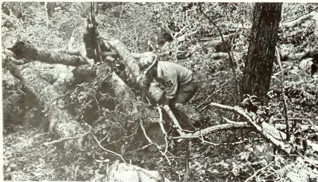
A forester hooks a cable to a log deep in a valley to demonstrate how the cable yarder lifts trees from difficult locations, while an operator controls the gasoline engine.
