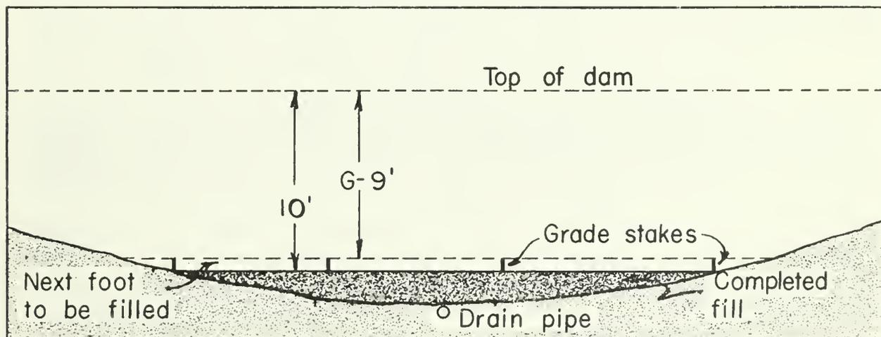
—Diagram is a side view of incomplete dam, showing grade stakes set for the next foot of fill. “G” is the remaining height of dam to be built above the established 1-foot grade stakes.
