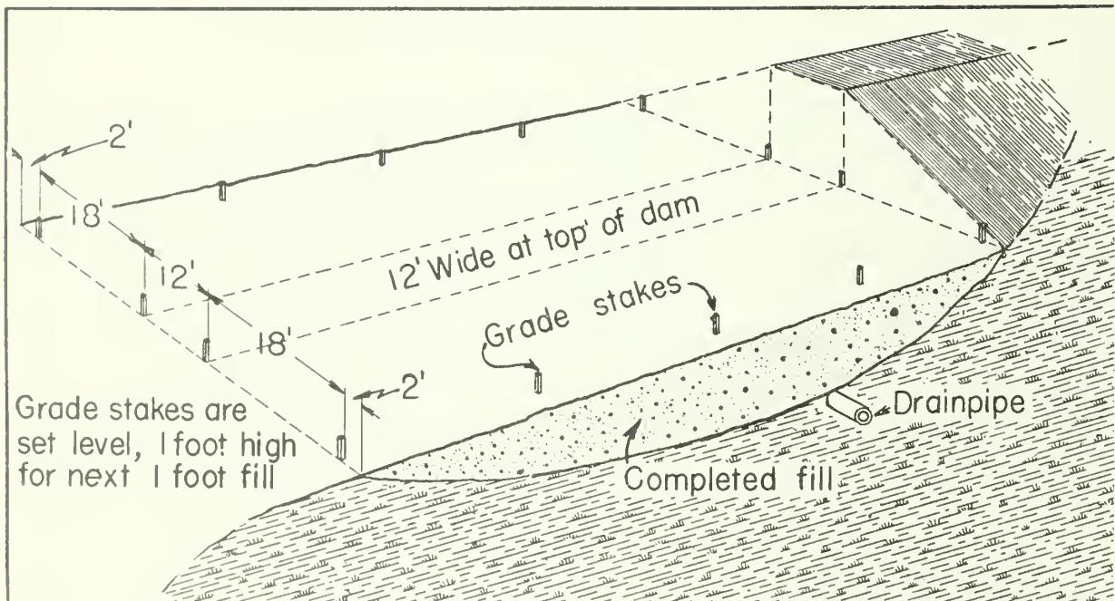
Perspective view of Figure 14 shows position of stakes on fill.
