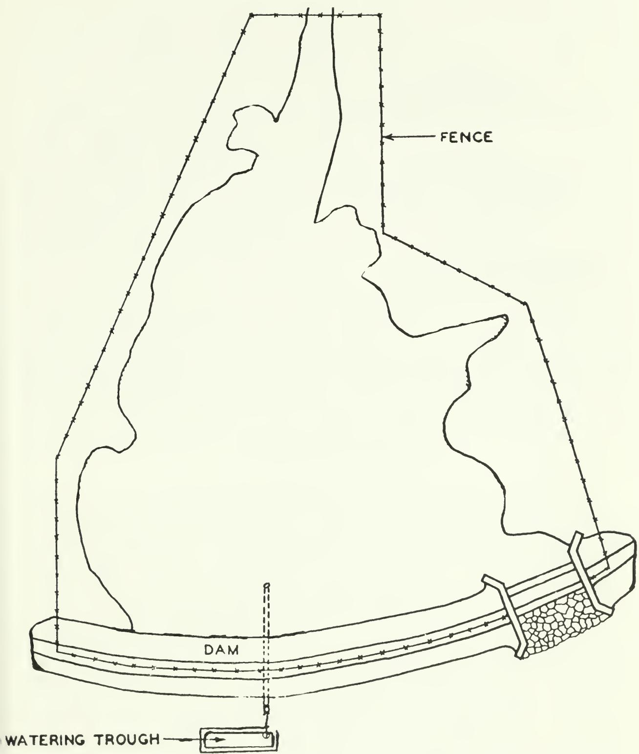
—Drawing of assumed lake showing how pond should be fenced. Notice spillway is placed to side to release water sufficiently downstream to prevent water current from back washing levee.
