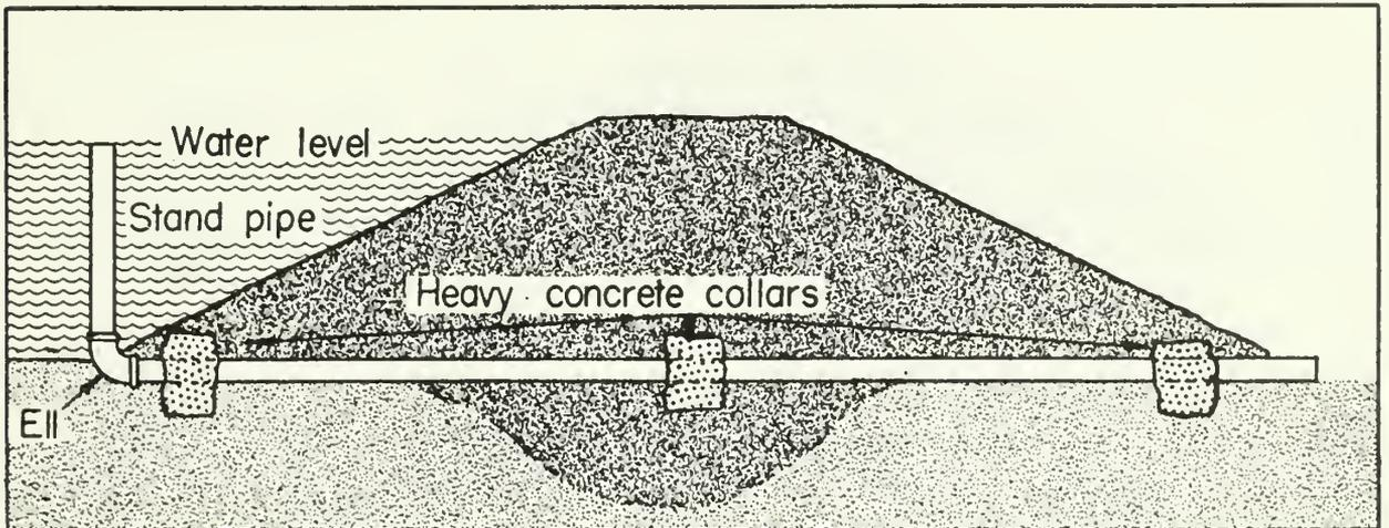
Cross-sectional diagram shows how threaded pipe with an ell may be used for a pond drain, eliminating the use of a valve. Heavy concrete collars must be placed at about 15-foot intervals to prevent the pipe from turning and prevent water from seeping along side of the pipe.
