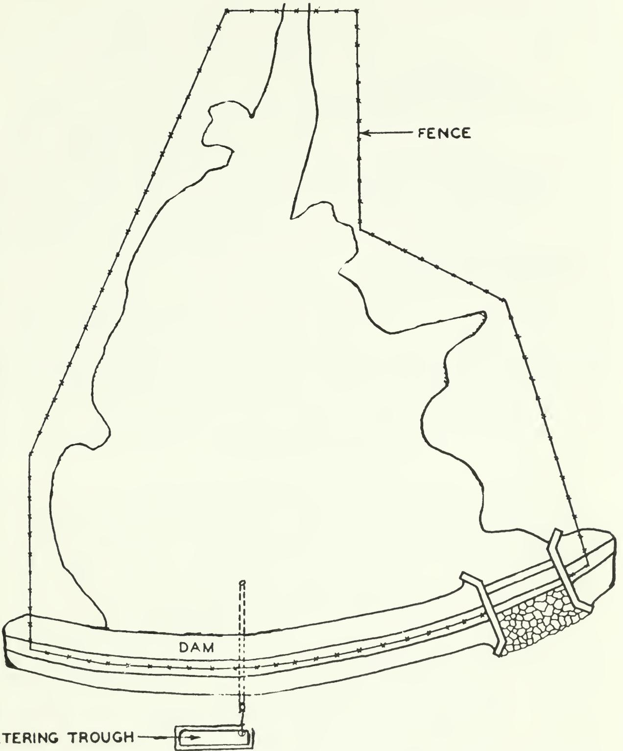
—Drawing of assumed lake showing how pond should be fenced. Notice spillway is placed to side to release water sufficiently downstream to prevent water current from back washing levee.
