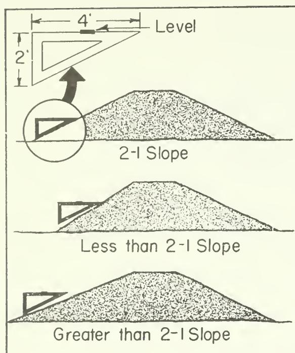
—Diagram shows use of home-built triangle-level that may be used in maintaining the 2-to-1 slope.
