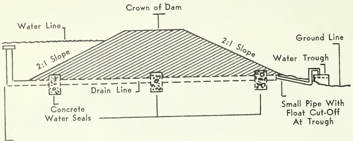
Ell Standpipe Used To Catch Water Near Surface It Can Be Turned Downward If Water Level Is Lowered
