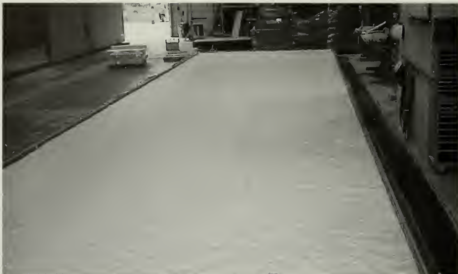
Figure 6. Taken at the composite manufacturer, this photo shows layers of fiberglass arranged around the deck core and placed in the mold. The mold was then infused with a resin that sealed the layers into a one-piece panel. Photo: Hayati Catbas, Hardcore Composites.
