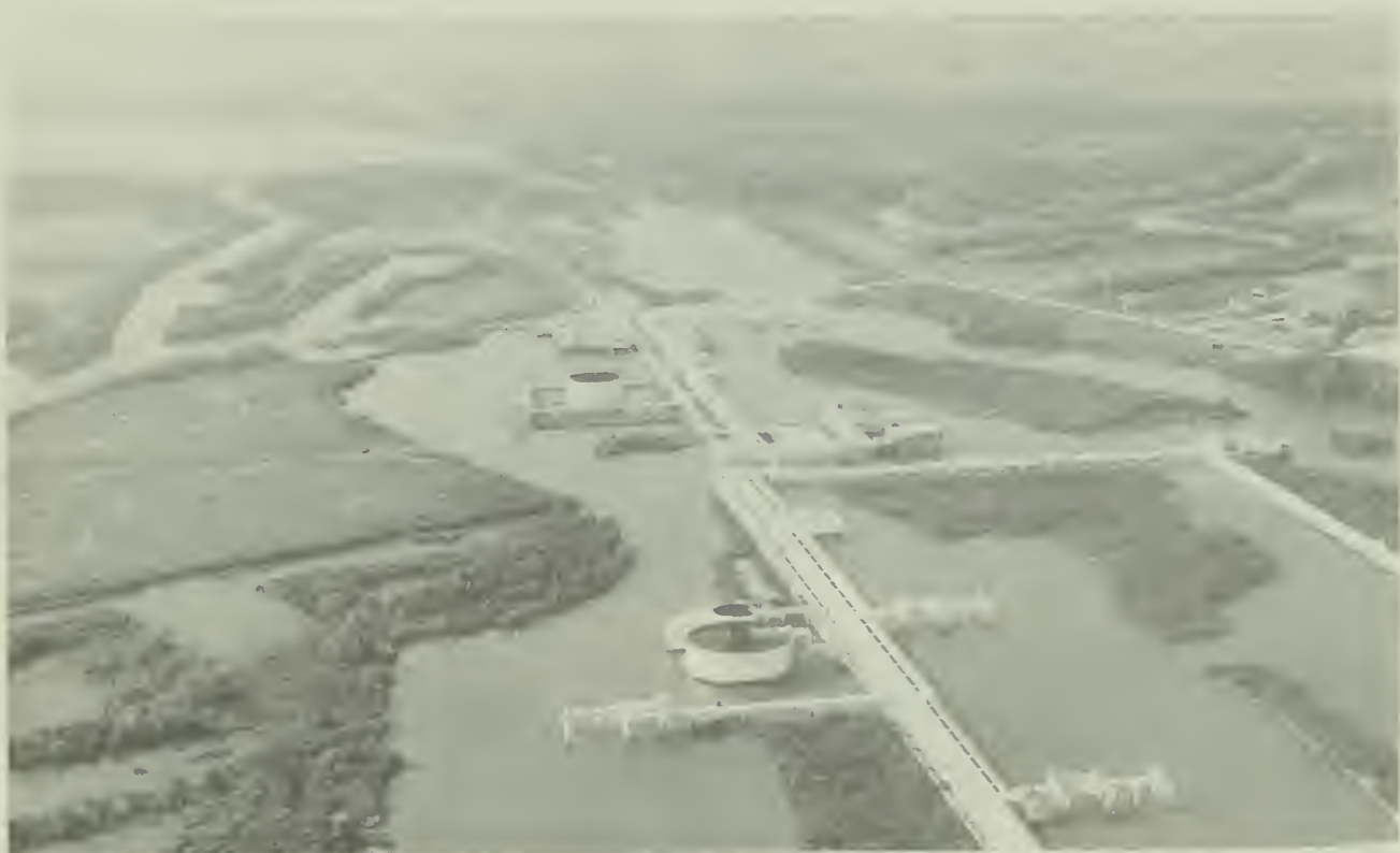
Figure 2. The oil storage facility for the nation's only superport is constructed in a salt dome in the middle of a Mississippi delta brackish marsh. The maze of pipes is the primary aboveground expression. An old oilfield also sits atop this submerged salt dome as shown by the network of tree-lined oilwell access canals (Photograph by Robert Abernathy).
