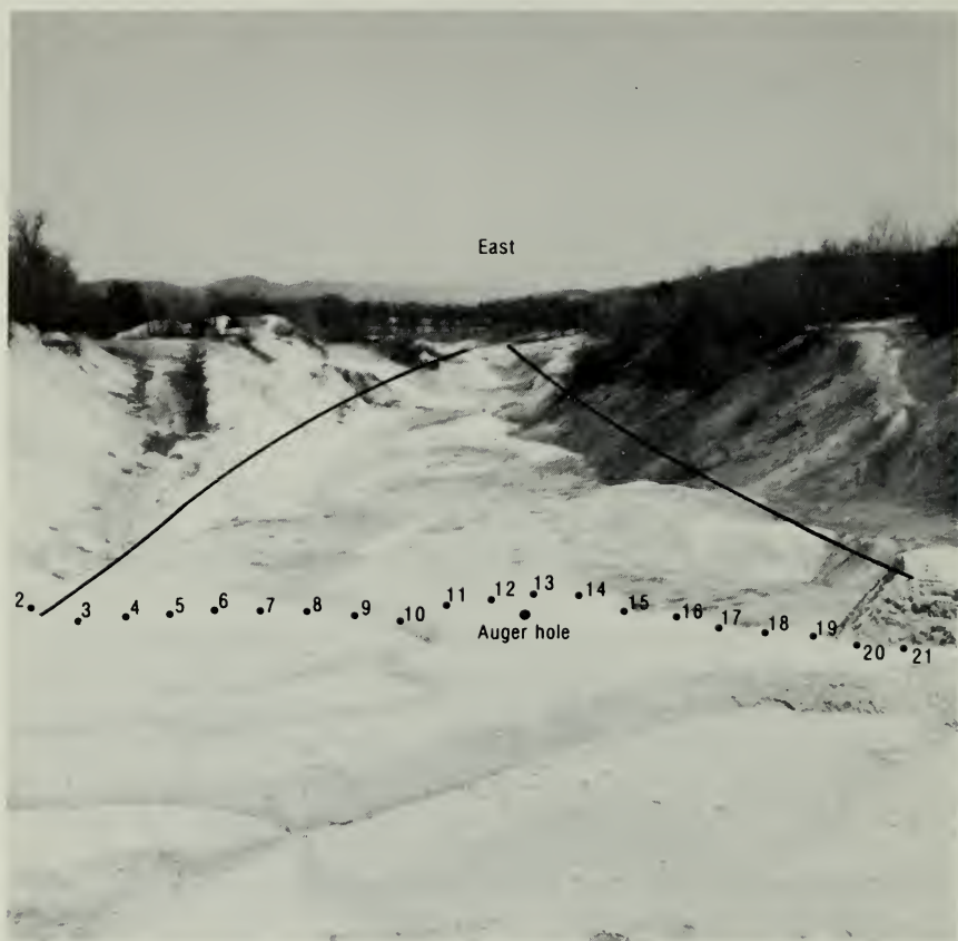
FIGURE 5.—Clay mine in the Stormstown pit, Centre County. The view is looking east and shows the north and south limits of the pit and the location of the auger hole. Numbers refer to sample locations.
