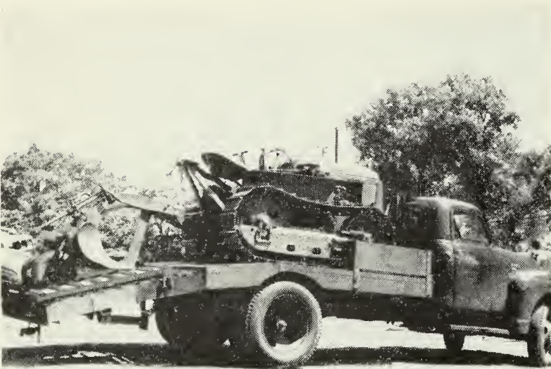
Light suppression plow and tractor unit utilized in fire suppression in upper Piedmont and mountain areas.
