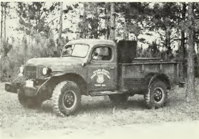
Rugged, low-geared power wagons equipped with power water pumps and tanks for fire fighting in Coastal Plain and lower Piedmont.
