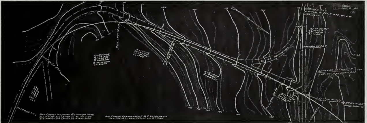
Figure 1.39. Plan of Kebo Mountain Road Extension showing the alignment along existing roads and the location of the bridge carrying State Route 3 over the motor road. (Federal Works Agency, Public Roads Administration, Project 6A3-8A1, Sheet 4 of x, September 1939)
