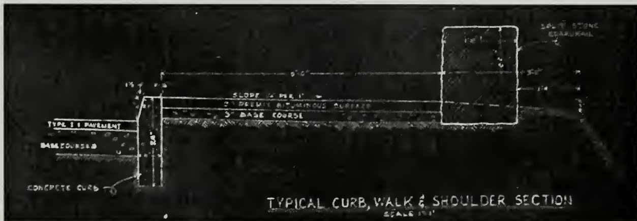
Figure 3.37c. Detail of paved walkways with curbs at the Sand Beach parking area. (U.S. Department of Commerce, Bureau of Public Roads, Project 43A1, Sheet 6 of 23, February 1953)
