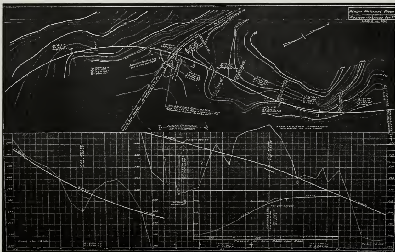
Figure 3.4. A sheet from the Paradise Hill Road drawings, at the bridge over New Eagle Lake Road, showing alignments and grades. (Federal Works Agency, Public Roads Administration, Project 10A1, Sheet 8 of 77, April 1940)
