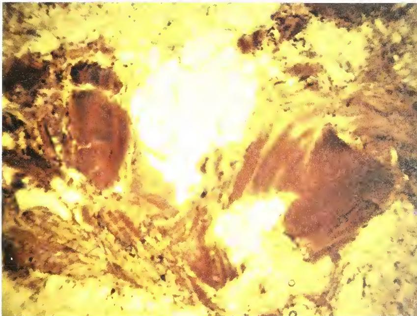
Figure 8.--Weathered biotite grains exhibiting iron oxide staining of adjacent feldspars and partial alteration of biotite to iddingsite and smectite.
