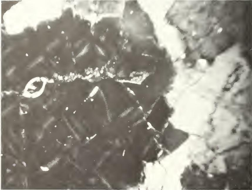
Figure 18.--Dark area at left is a large quartz grain near extinction (no transmission of polarized light). Light lines are strain induced and bound domains of crystal lattice deformation. This results in an undular extinction pattern when the microscope stage is rotated. Magnification = 100X; crossed nicols.
