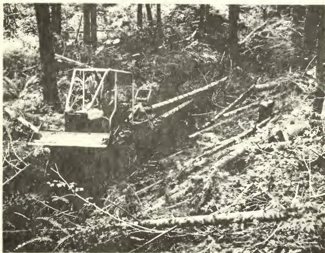
Figure 5.--The Tree Farmer represents an improved method of skidding, requiring less labor and allowing a greater efficient-skidding radius.
