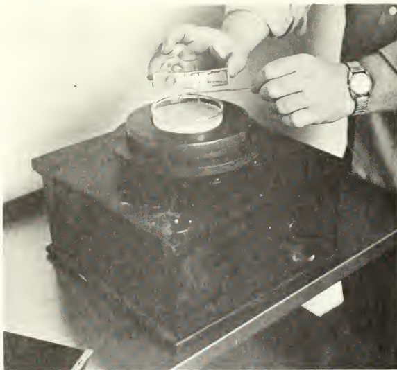
Figure 1...Spreading an aliquot of soil-water suspension on agar surface with aid of glass rod and modified spring-operated phonograph turntable.
