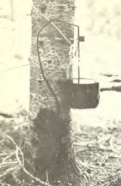
Figure 1.--Apparatus for injecting dye into study trees.
