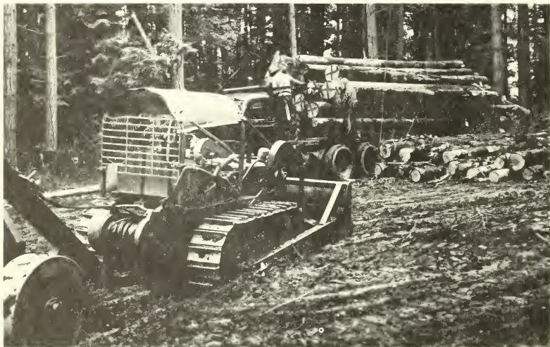
Figure 4.--The crawler tractor is not well suited to thinning in small timber and light cuts.
