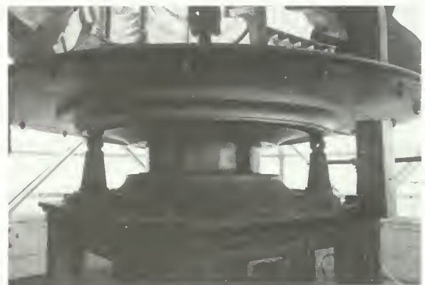
Figure 36. This c. 1926 lens was designed to be AC powered; the original lens jacks are still in place. The three jacks (the third is obscured by the brass bearing cover) were used to lift the lens assembly so that bearings could be serviced.
