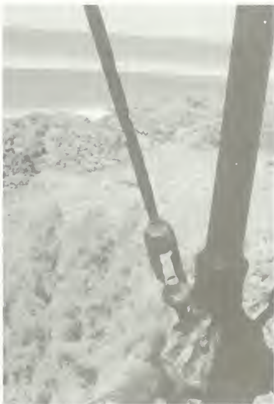
Figure 16. As corrosion attacked this steel turnbuckle, wind and airborne sand eroded away the flaking rust.
