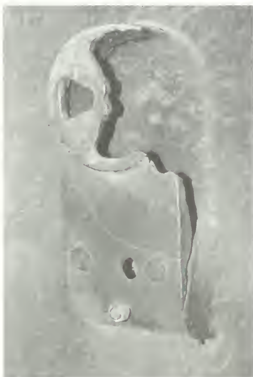
Figure 14. Nearly 30% of this ventilation shroud has been lost to two forms of abrasion: first, sand or grit blasting abraded away a majority of the material; second, human touch has smoothed the once rough surface.
