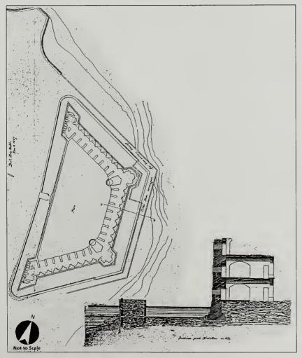
Figure 1.29: Plan and section drawings made in 1857 showing the moat and cobble filled timber cofferdam to the east of the fortress built to allow construction of the permanent stone seawall. Note that the dock has not yet been built at the bulkhead visible at the top of the drawing. RG 77, Dr 43, Sht. 46, Cartographic Division, National Archives II, College Park, Maryland, annotated by SUNY ESF.
