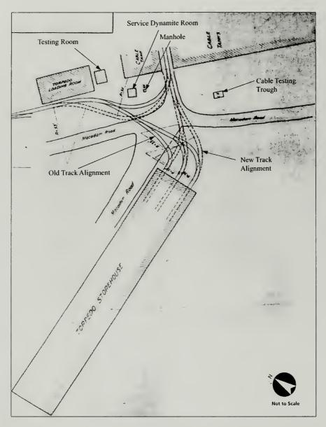
Figure 1.59: Plan made in 1921 showing the preexisting (solid lines) and the proposed 1921 (dashed lines) alignment of the mine railway at the Torpedo Storage Building (noted as Torpedo Storehouse). National Archives, reproduced from Ingrid Wuebber and Edward M. Mońn, "Phase 1A Archeological Investigation Rehabilitate Battery Weed Seawall and Dock" (Unpublished report prepared for the National Park Service by URS Corporation, 2006), annotated by SUNY ESF.
