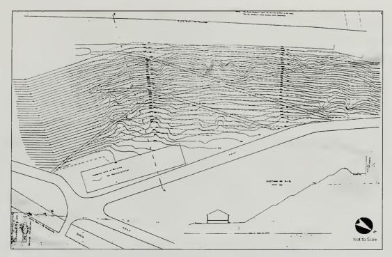
Figure 1.46: Detail of an 1892 survey illustrating the diagonal walks built after 1886 on the engineered slope, showing route that extends to either side of the proposed Torpedo Storage Building at the base of the slope. The plan also shows the former natural contours prior to grading in c.1873. RG 77, Dr 43, 90-2, 1892, Cartographic Division, National Archives II, College Park, Maryland, annotated by SUNY ESF.
