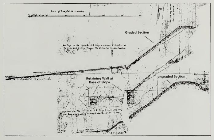
Figure 1.26: Two sections taken across the slope above the new Fort Richmond showing the existing slope and the area to be graded, 1848. The drawing also shows the planned retaining wall to be constructed at the base of the graded area. RG 77, Dr 43, Sht. 12, Cartographic Division, National Archives II, College Park, Maryland, annotated by SUNY ESF.
