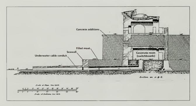
Figure 1.53: Section drawing accompanying plan view (Figure 1.52) showing the concrete additions (hatched areas) built around the original granite bastion within the dewatered moat, and the cable conduit that extended into the Narrows. RG 77, Dr 36, Sht. 100-5, 1887, Cartographic Division, National Archives II, College Park, Maryland, annotated by SUNY ESF.
