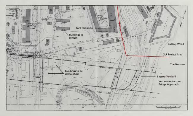
Figure 1.63: Plan drawn in 1959 showing buildings to be demolished (white fill) on approaches to the Verrazano-Narrows Bridge at the eastern end of Fort Wadsworth. The area north of Battery Weed was not included on the plan. Triborough Bridge and Tunnel Authority, "Replacement of Facilities Displaced by the Narrows Bridge, Fort Wadsworth Water Distribution System Area 3," 1959 updated to 1963. Gateway National Recreation Area Archives, Fort Wadsworth, annotated by SUNY ESF.
