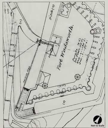
Figure 1.51: Detail of the 1886 plan (Figure 1.36) illustrating the dewatered moat (noted as "Ditch" on plan) and reservoir created at the southwest bastion of Fort Wadsworth (Battery Weed). Water was carried from a suction pipe along the moat wall to a pump in the guardhouse. These changes to the moat were probably the first steps in development of the mine defense system. RG 77, Dr 41, Sht. A, Cartographic Division, National Archives II, College Park, Maryland, annotated by SUNY ESF.
