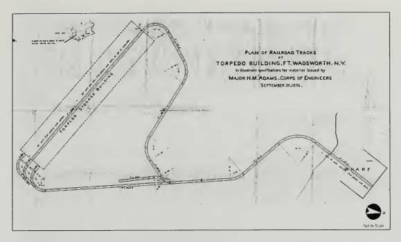
Figure 1.54: Plan drawn in 1896 showing the Torpedo Storage Building and mine railway constructed to move mines and cables from the building to the wharf (north stone dock). At the upper left is a perspective section of the rails. National Archives, RG 77, Dr 43, Sht. 90-11, 1896, Cartographic Division, National Archives II, College Park, Maryland, annotated by SUNY ESF.
