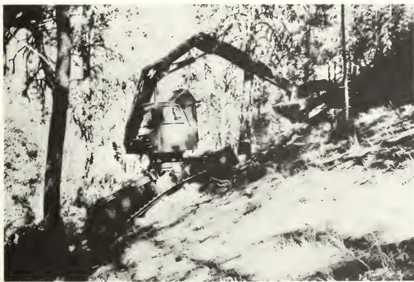
Figure 5—Track-mounted steep-slope feller-buncher equipped with self-leveling platform carrying a boom-mounted tree shear that can accumulate sheared stems preparatory to depositing them in a bunch.
