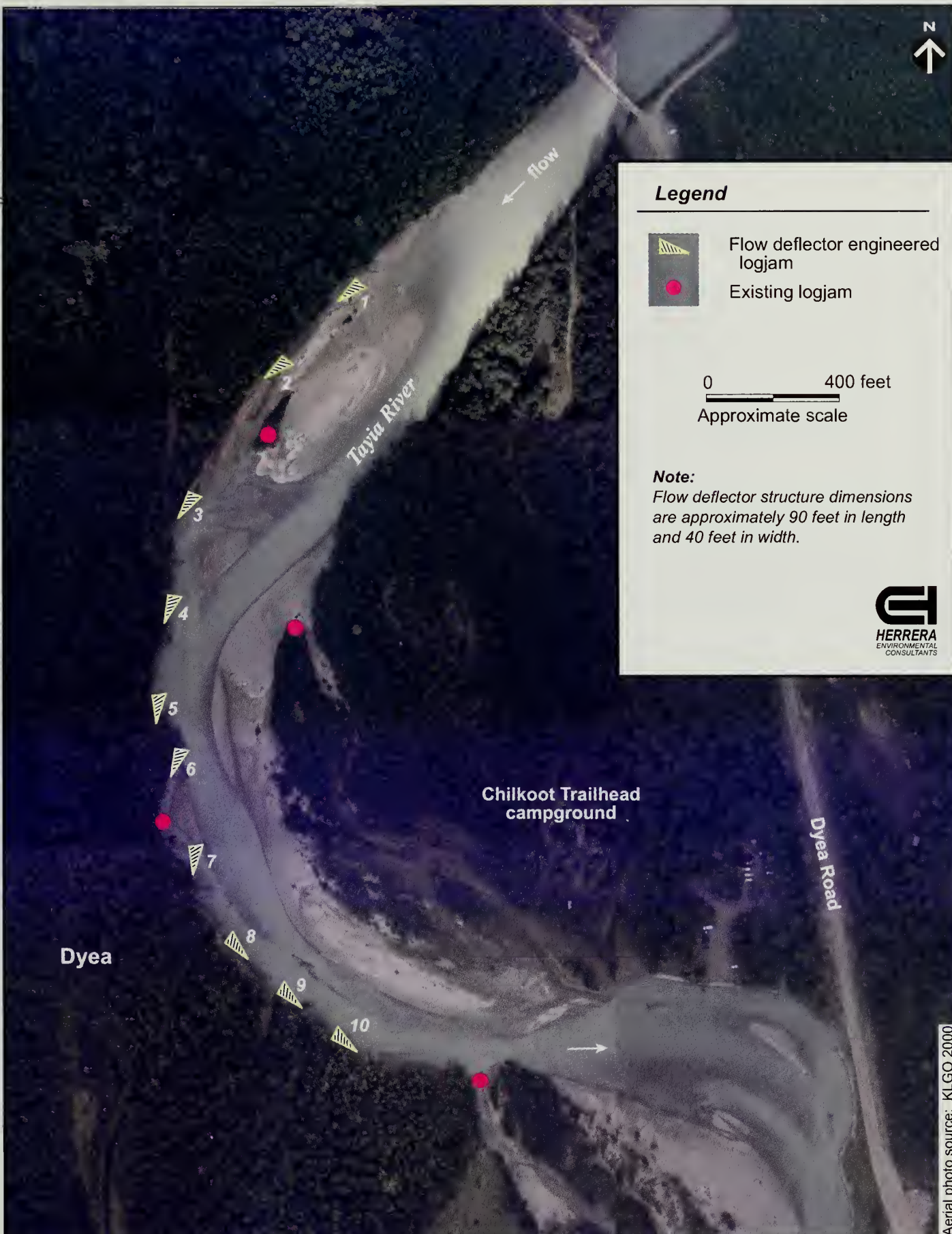
Figure 11. Conceptual plan view of flow deflector engineered logjams for option A.
