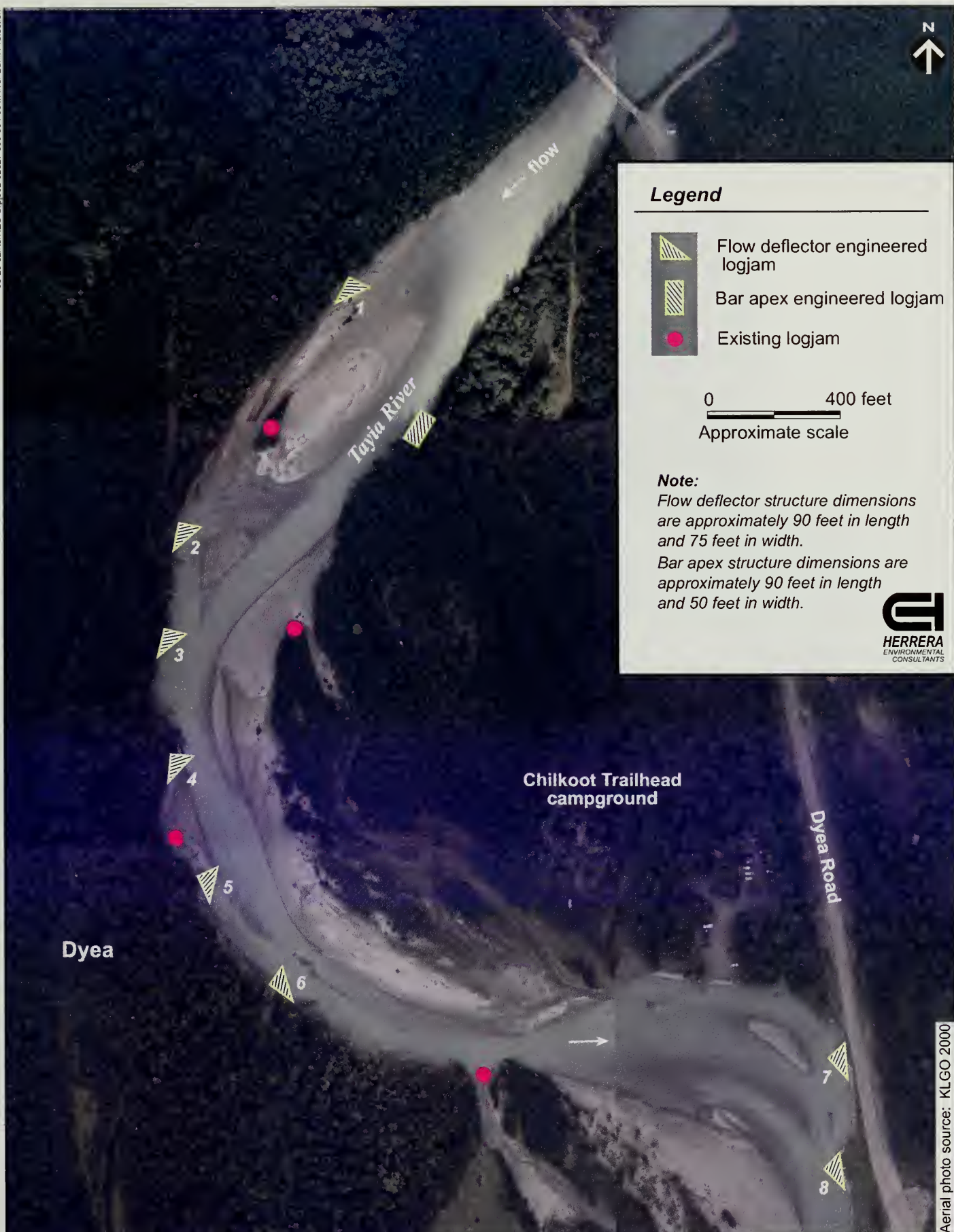
Figure 12. Conceptual plan view of flow deflector and bar apex engineered logjams for option B.
