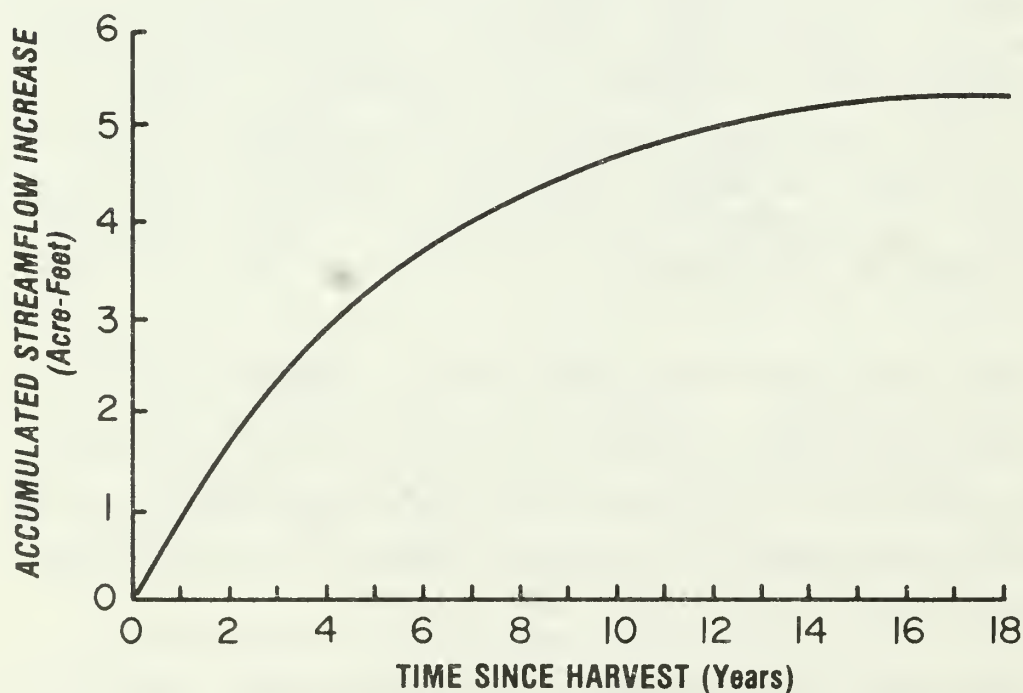
Figure 22.--Accumulated increases in streamflows estimated for the Big Ivy forest, by time since harvest of 100 percent of the basal area of a stand; average slope is about 14 percent and faces west.
