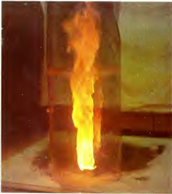
Figure 1.—A laboratory-created fire-whirl in a plastic chamber. The plastic is joined along the seam with nut-bolt bracing that leaves a 1/2-inch space along the entire length, allowing air to enter. The air becomes a generating eddy as it is forced to spin around the inside of the chamber gaining vorticity. Lighter fluid in the small cup provides the fuel source. Intense heat generated by the whirl has caused the inexpensive plastic cylinder to buckle. The direction of spin can be reversed by inverting the cylinder.
