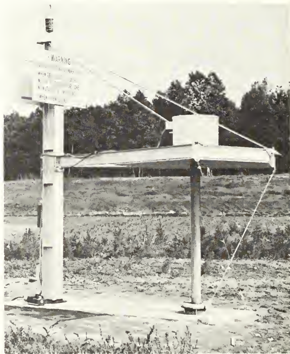
Figure 10. — Gamma field radiation source support and operating mechanism. The radioactive source capsule, containing 1,500 curies of Cesium 137 , is elevated in the tube to a position just below the sky shield to irradiate tree seedlings planted in the area around the source.
