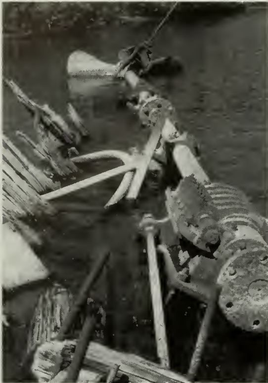
Figure 5.34. View west of E. C. Waters' propulsion system. The engine bed is in the foreground, the thrust bearing is in the middle foreground and the propeller shaft and the propeller is in the background. NPS photo by John Brooks.
