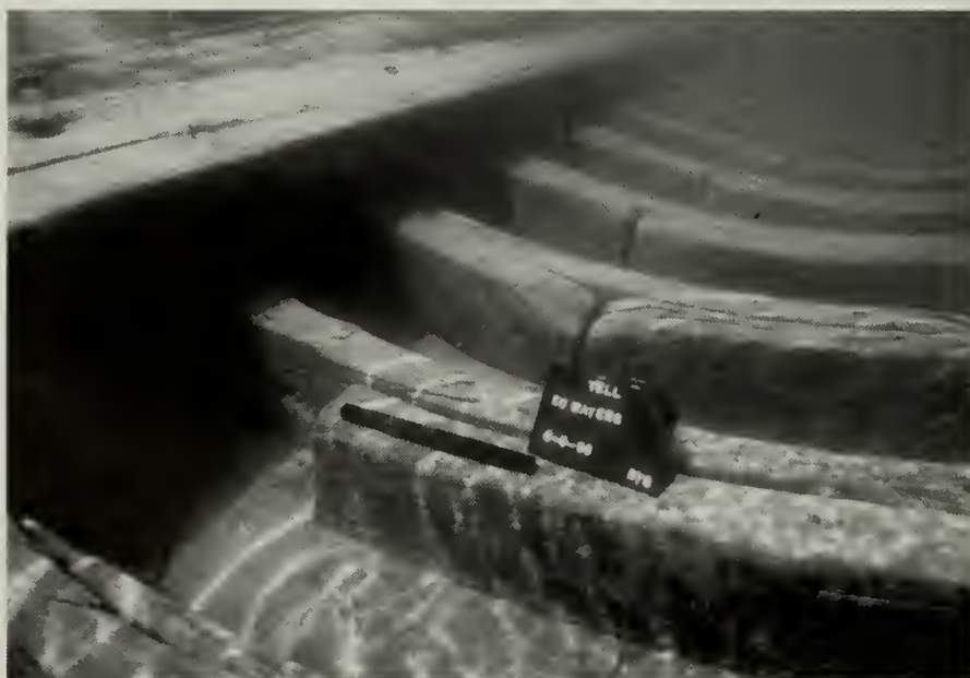
Figure 5.29. E. C. Waters' frames. View aft of paired frames with butt joints in the wreck's forward port section. The main and sister keelsons overlay the frames in the upper left. Scale = 1 foot. NPS photo by Brett Seymour.
