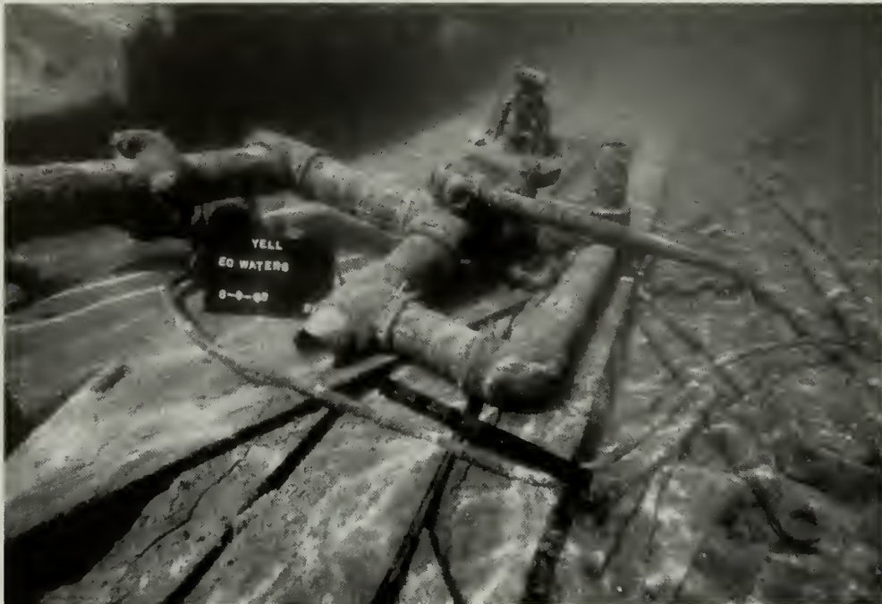
Figure 5.44. View aft along port midships showing feed water intake piping (foreground) and globe valve (background). Scale = 1 foot. NPS photo by Brett Seymour.
