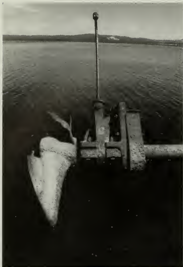
Figure 5.41. View north, starboard side of adjustable stern bearing assembly (center) and propeller (left). NPS photo by John Brooks.
