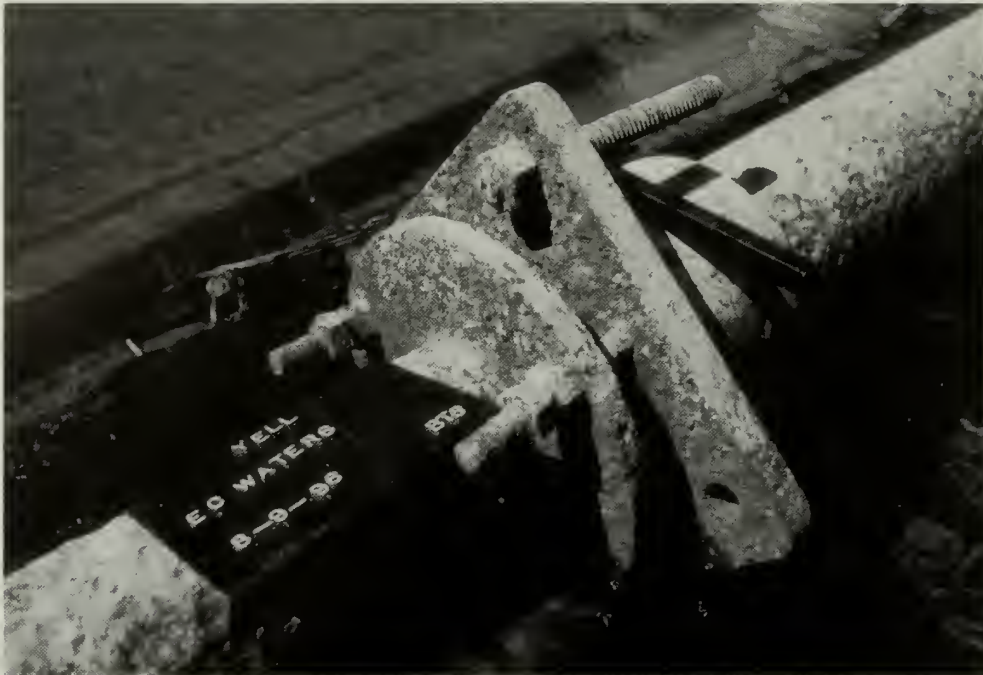
Figure 5.39. View southwest of forward end of stern tube stuffing box and gland. Note large bolt on top that secured the shaft to the stern deadwood (now missing) through which it passed. Marked section of scale = 6 inches. NPS photo by Brett Seymour.
