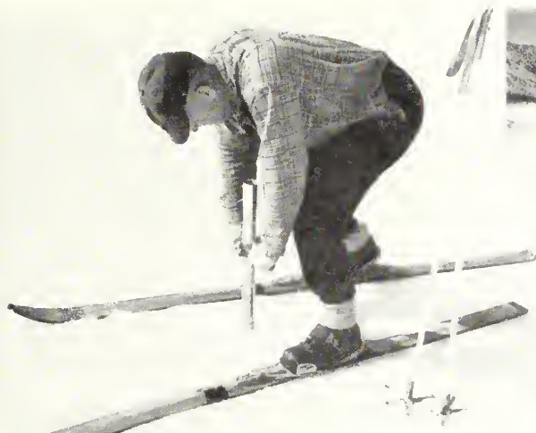
SECRETS IN THE SNOW are ferreted out with a sampling tube (above). Surveyors use various means of transportation over the snow courses (inset). Both photos by the Soil Conservation Service, United States Department of Agriculture.
