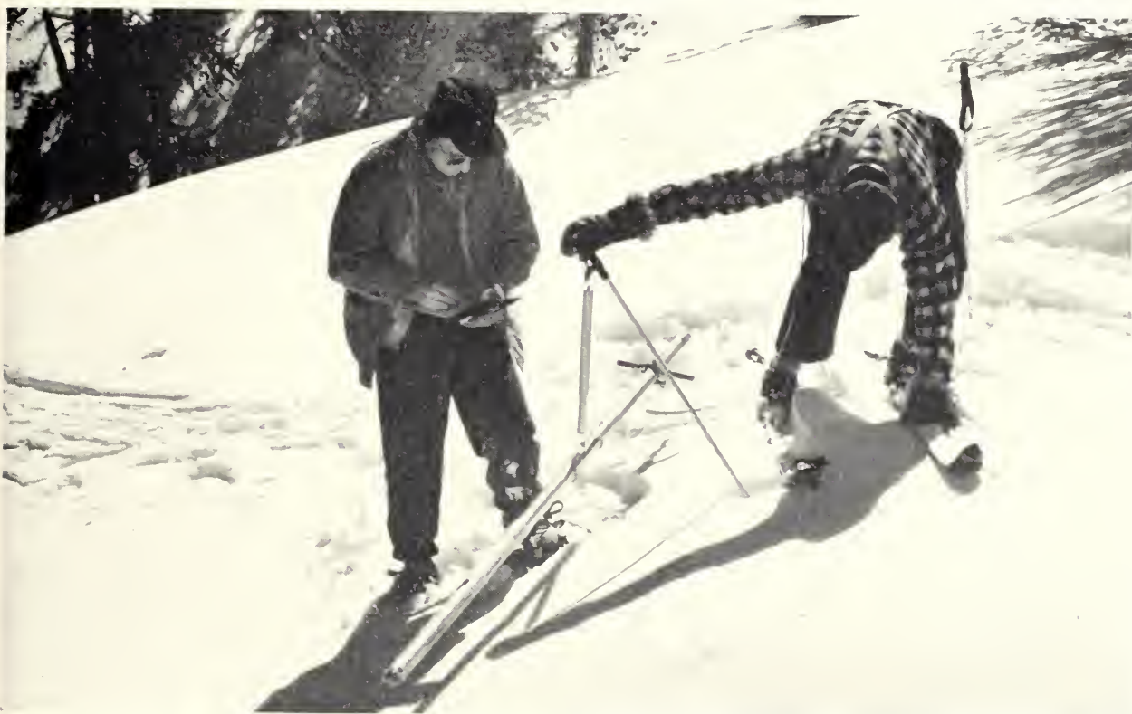
WHEN THE SNOW MELTS, how much water will run to the streams and fill the reservoirs? Snow surveyors find out by carefully weighing the hollow aluminum tube with its core of snow on specially calibrated scales. Photo by Robert Branstead, courtesy of the Soil Conservation Service, United States Department of Agriculture.
