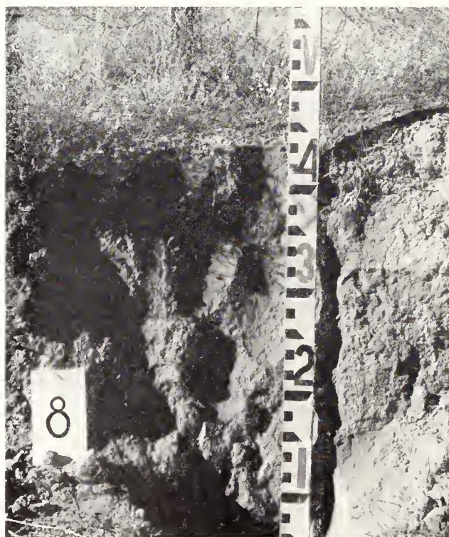
PROFILE OF PRODUCTIVITY. —At left, class 1 land in the Quincy Basin—a deep silt loam. Below, class 3 land (3-5) of the West Wahluke Slope—coarse sand and gravel close to surface. Note Saddle Mountains in the background. Markers show depth of pit, numbers indicate location, according to land classifier's map. Both photos by F. B. Pomeroy, Region 1 photographer.
