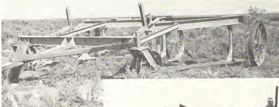
RAY SHERWOOD'S BRUSH CLEARER. —At left, the thin sharp blades which slice the brush off 2 or 4 inches below the ground. Below, the special rake, also designed by Sherwood, which does a good job of windrowing the sagebrush. Both photos by O. L. Kime.
