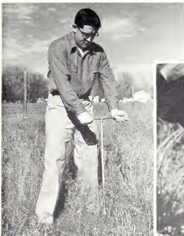
WHAT KIND OF SOIL? —The soil auger can be used to obtain samples for determining soil texture as well as finding out the moisture holding capacity of the soil, and when to apply irrigation water. Photos by Phil Merritt, Region 1 photographer.
