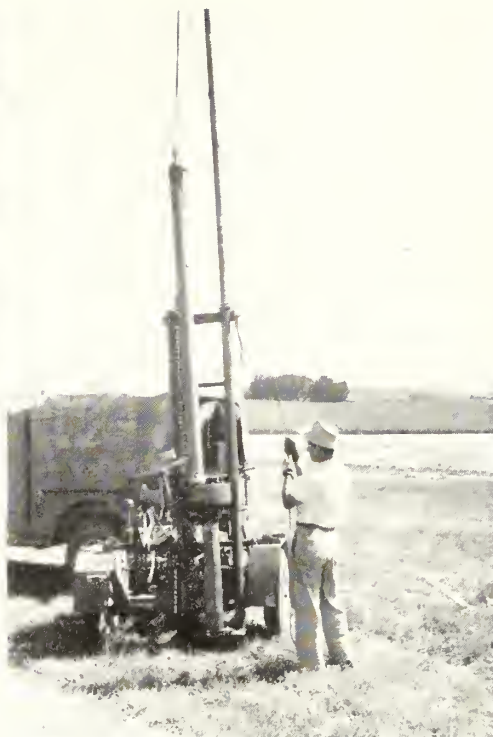
ON THE GROUND. —Special machines carve cylinders of undisturbed soil for analyses or to observe soil characteristics and permeability, especially in relation to drainage. Photo courtesy of Oregon State College.
