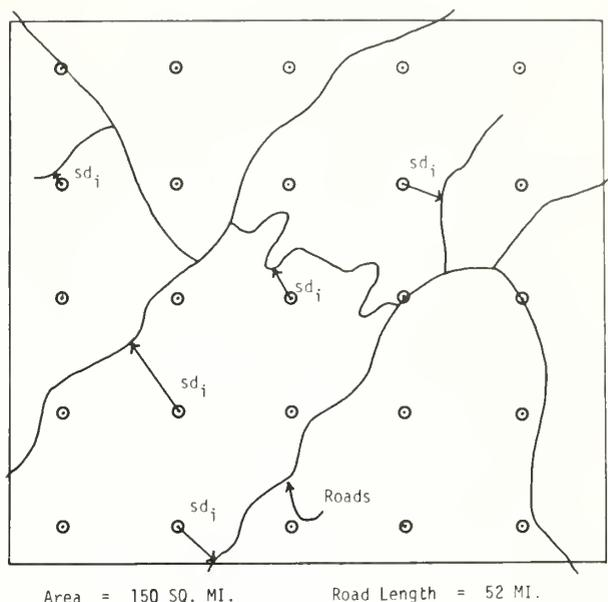
Figure 2. - Plane, irregular road net with dot grid overlay, and examples of  $sd_i$ .
