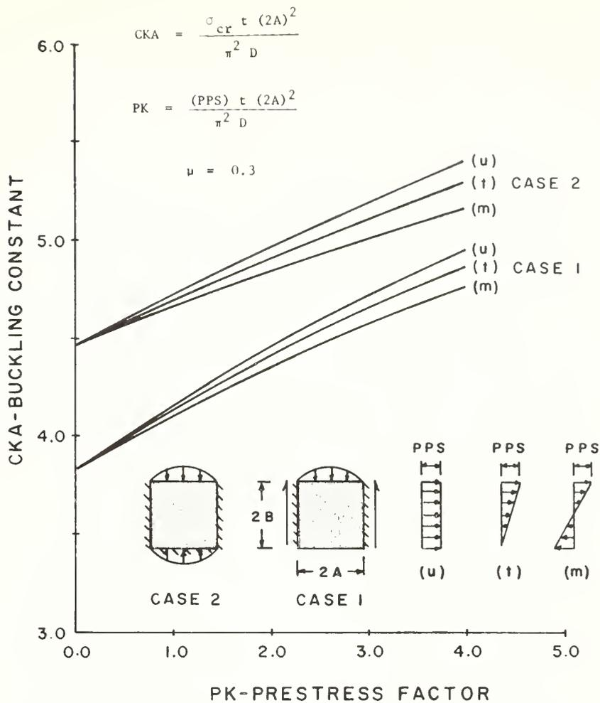
Figure 7.--Plot of buckling constant vs. prestress factor!
