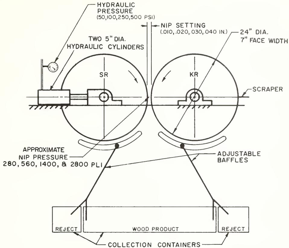
Figure 2. - Simplified compression debarker and machine variables.
