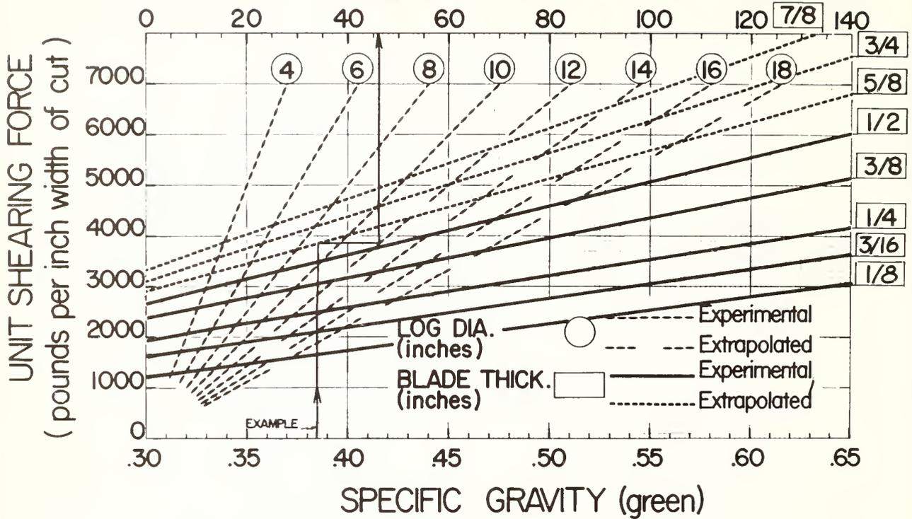
Figure 9.--Nomograph to estimate shearing force for different blade thicknesses.
