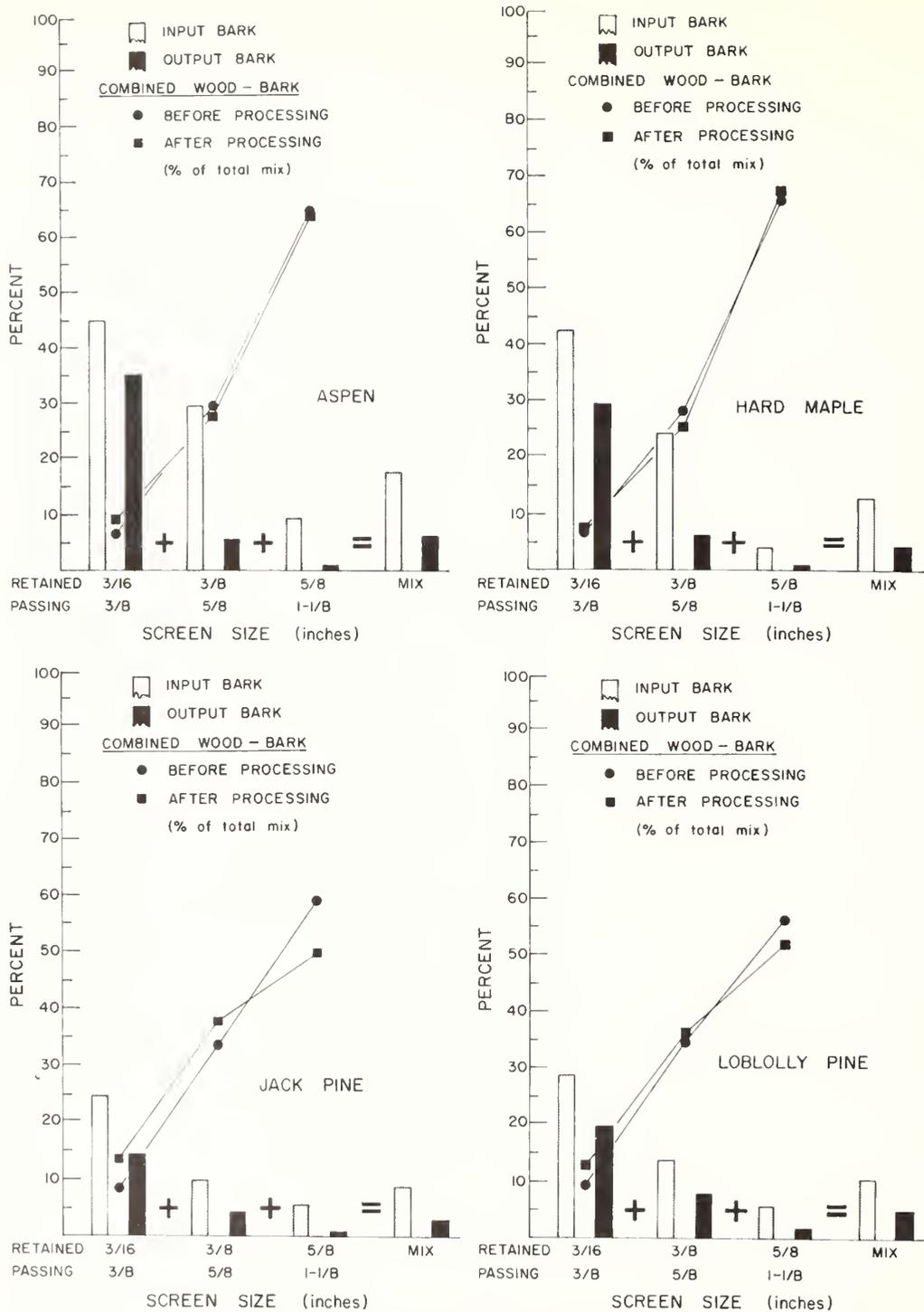
Figure 4. - Size breakdown and bark content before and after compression debarking.
