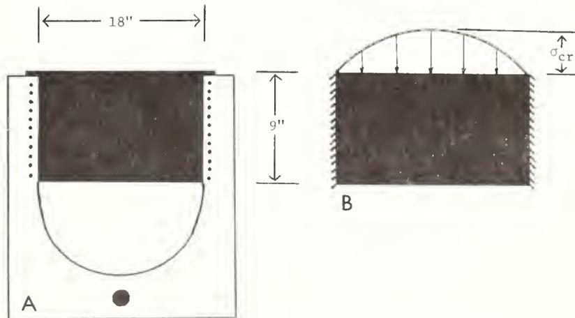
Figure 8.--Assumed shear blade configuration and simplified rectangular plate which most closely approximates this configuration. (For case A:  $t = 3/8$  inch,  $E = 30 \times 10^6$  psi, and  $\mu = 0.3$ ; for case B:  $B/A = 0.5$ , and  $CKA = 2.81051$  (from fig. 4 case 1)).
