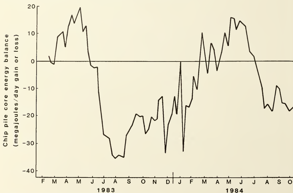
Figure 5—Chip pile energy balance based on outer pile temperatures, average ambient temperatures, and conductance.
