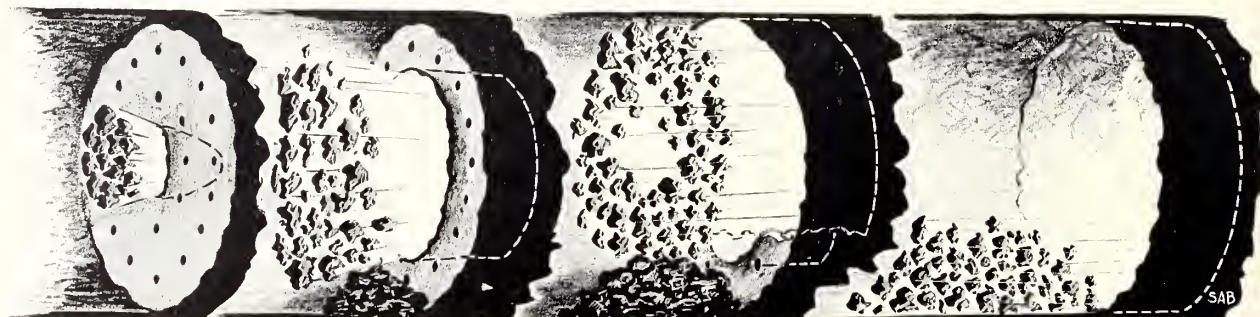
SLOW MOTION MOVIE showing the different phases in a dynamiting operation is represented in this stylized drawing. When the blasts were thrown off schedule at Duchesne by watery seams
