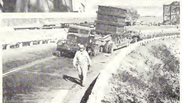
FRAMED IN STEEL the stark Arizona mountains rise in the background behind this 230-kilovolt switchyard at Davis Dam above. Above right: Close-up of crane using special sling to transport bushing for oil circuit breaker. The last lap (at right) truck and trailer en route to Davis Dam to deliver 92-ton, 45,000 kilovolt ampere main power transformer for first generator. All photos for this article by Phil Blew, Region 3 photographer.
