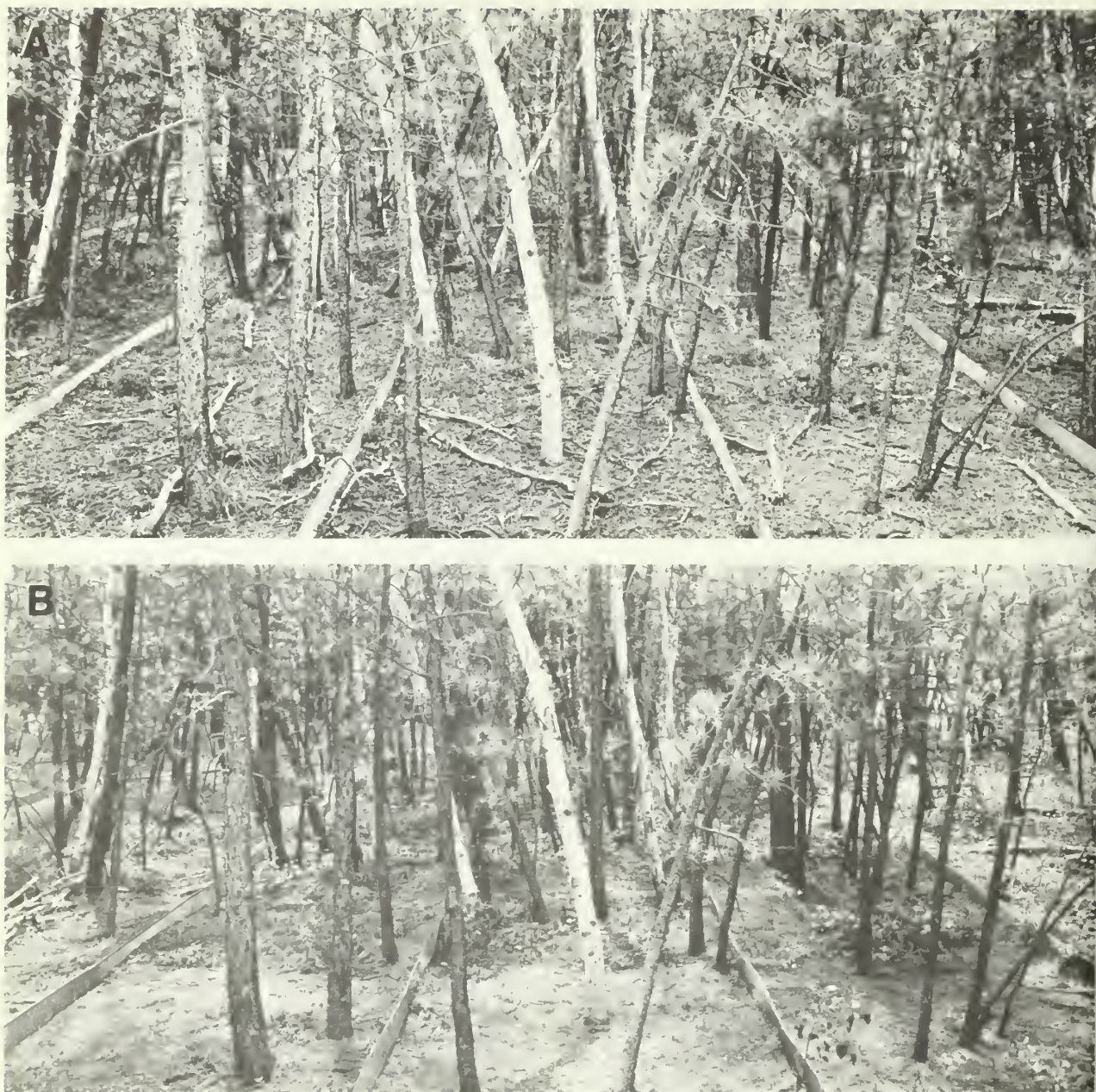
Figure 5.—Ponderosa pine runoff plots before (A) and after (B) litter removal.
