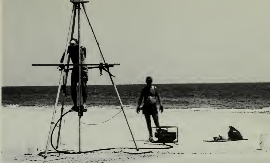
The Geologic Survey conducts vibrocoring on Georgia's coast to search for heavy mineral-bearing sands.
